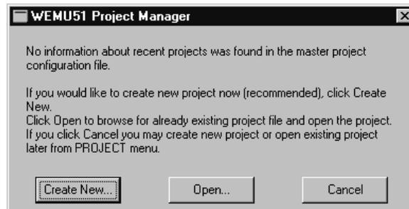
In order to begin working with the emulator you have to create a new project. The fastest way to create new project is by clicking the **Create New** button in the dialog box. This launches **Project Creation Wizard**.
