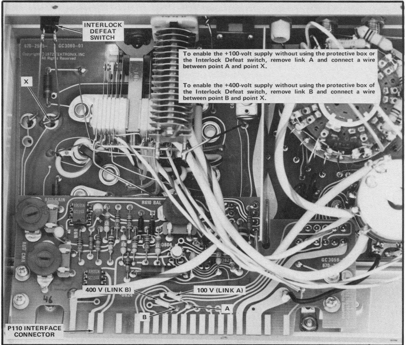
Fig. 3-2. 100 V and 400 V Interlock Defeat bypass option.
