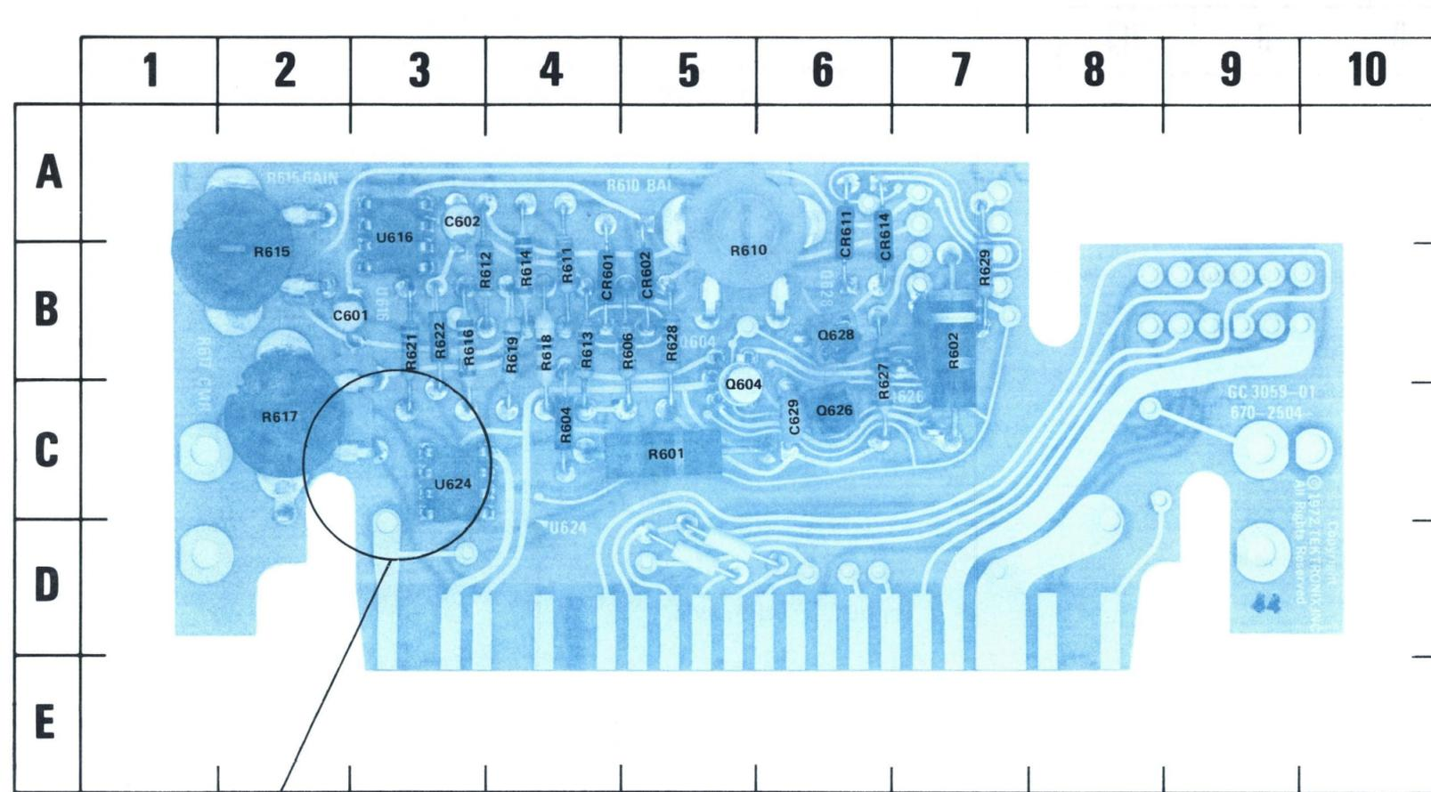
Fig. 7-1. A1 Pre-amplifier circuit board.
