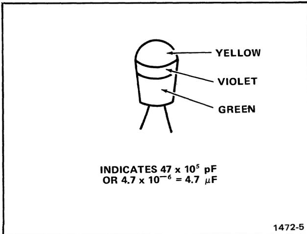
Fig. 4-2. Example of Electrolytic capacitor color code.
