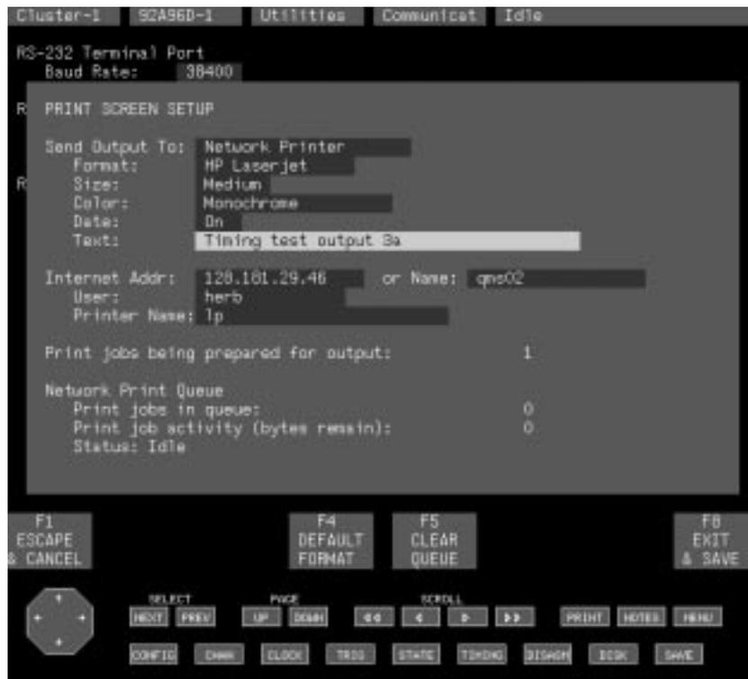
Figure 3–25: Print Screen Setup Overlay with Network Printer Selected
