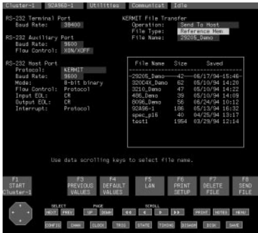
Figure 3-26: Communications Menu with the Kermit File Transfer Protocol
