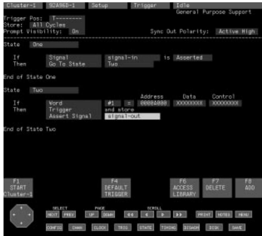
Figure 3–15: Trigger Program Using Signals
