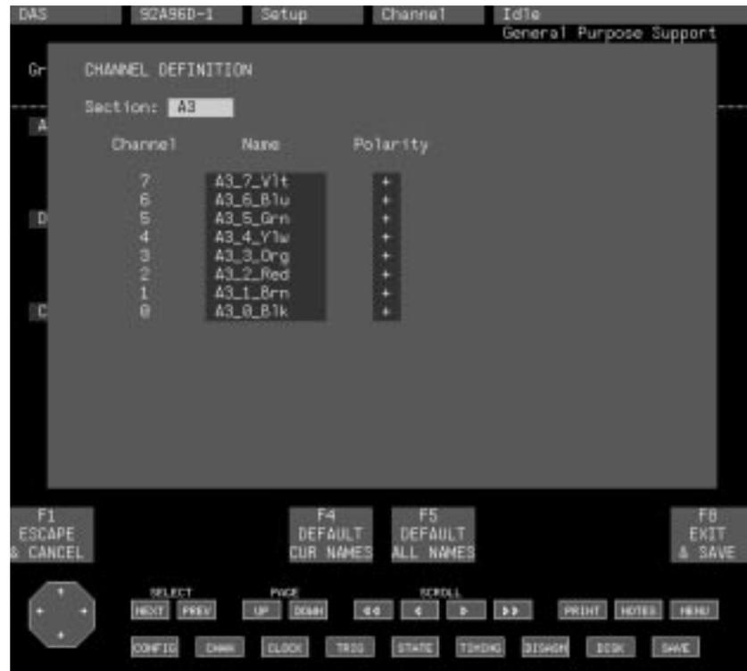
Figure 3–6: Channel Definition Overlay (Section Field Open)
