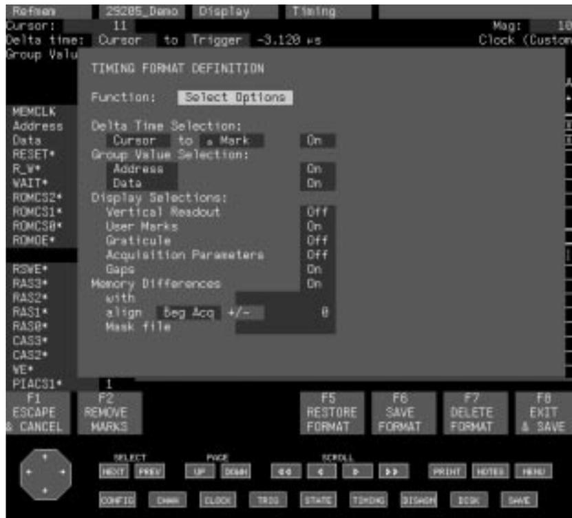
Figure 3–40: Timing Format Definition Overlay, Select Options Function
