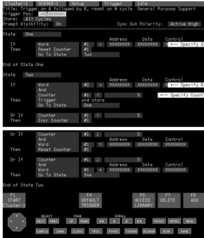
Figure 3–27: Complex Trigger Program (Trigger Menu)
