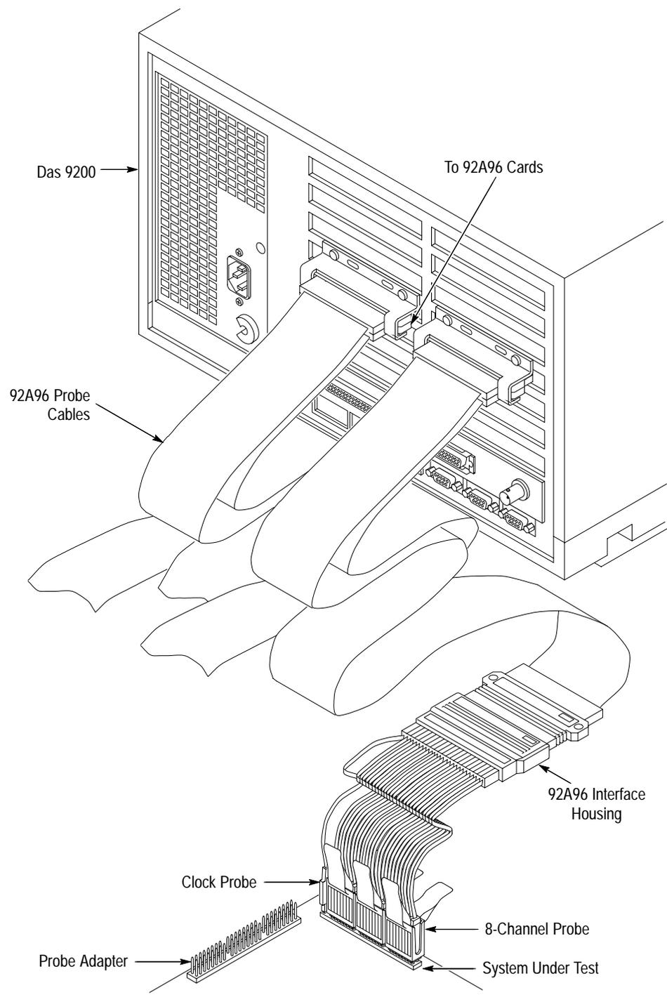
Figure 1-2: Connections to the System Under Test
