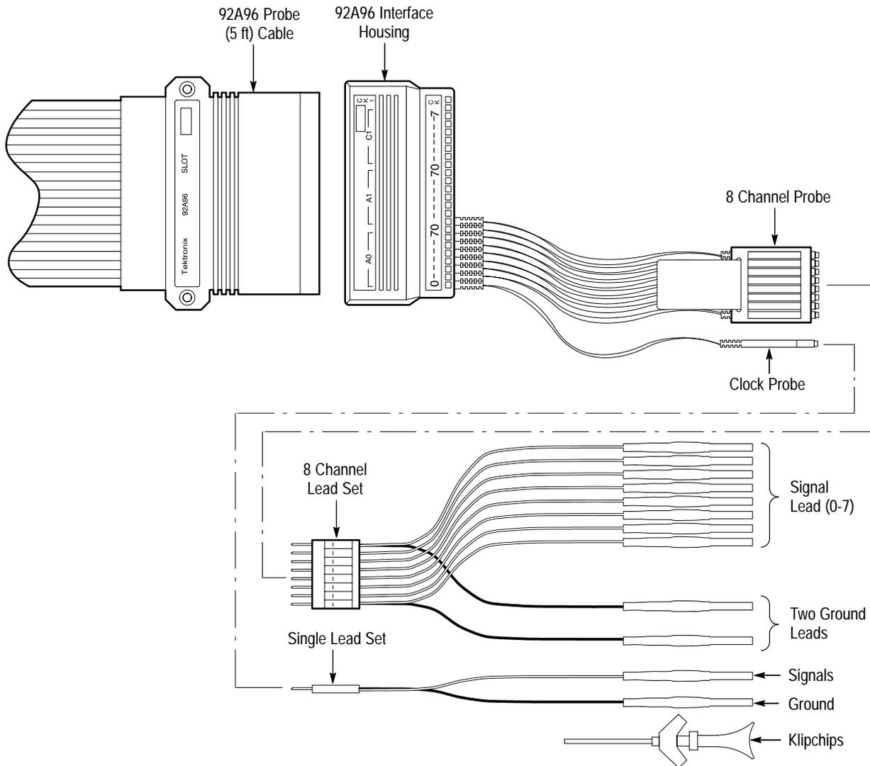
Figure 1–7: A 92A96 Probe Assembly and Lead Sets
