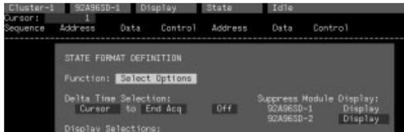
**Figure 3–34: Module Suppression Fields (State Format Definition Overlay)**
