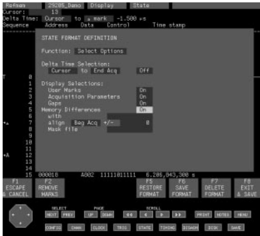
**Figure 3–33: State Format Definition Overlay, Select Options Function**
