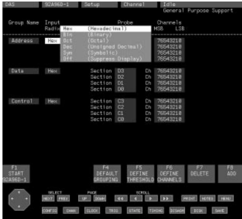
Figure 3-4: The Opened Input Radix Field (Channel Menu)
