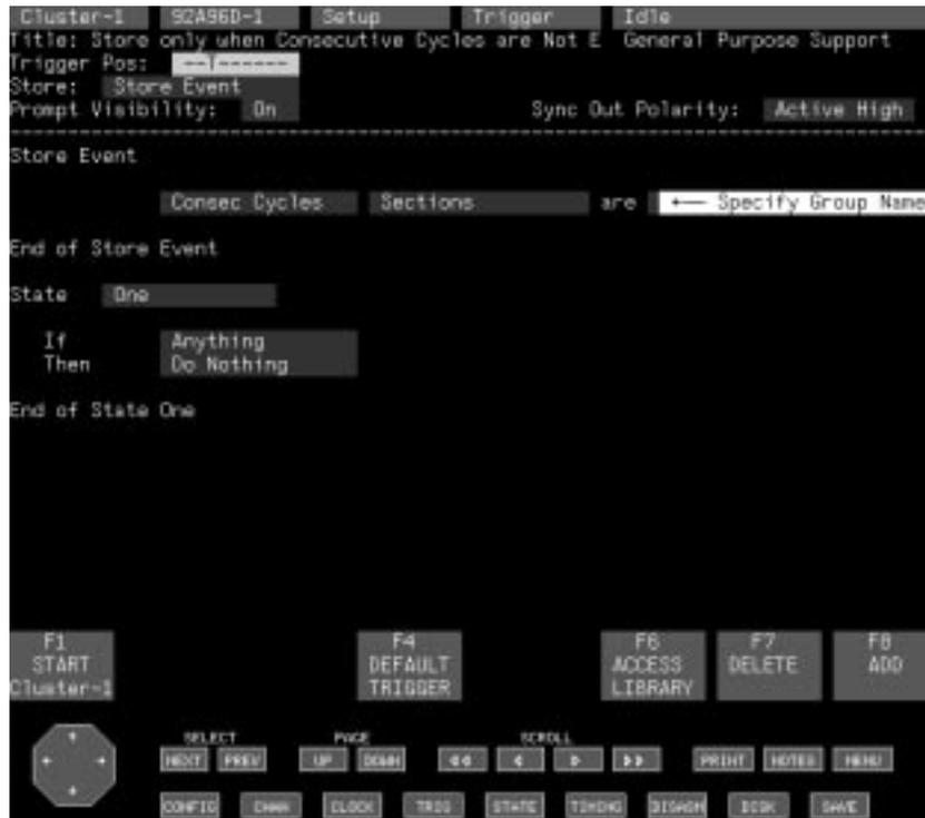
Figure 3–26: Simple Trigger Program (Trigger Menu)
