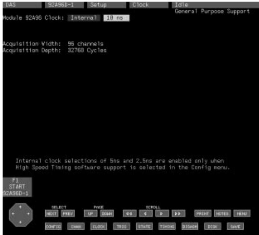
**Figure 3-7: The Clock Menu with Internal Clock Window Displayed**
