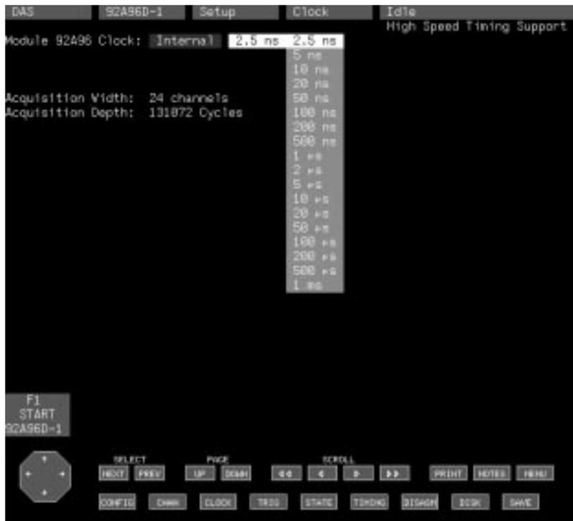
Figure 3-56: Clock Menu With Internal Clock Periods in High-Speed Timing Support
