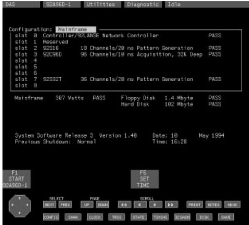
Figure 1–10: Diagnostics Menu Showing Results of Diagnostic Testing
