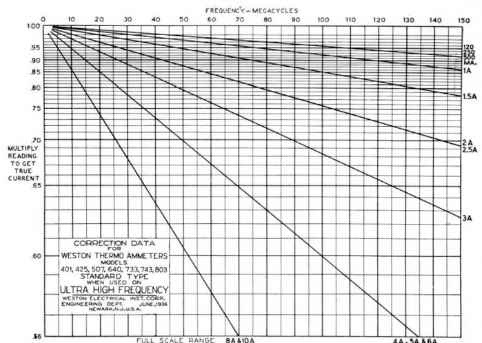
The data in the chart will not, of course, apply exactly to different designs of instruments but since the designs are rather severely limited by joint Army-Navy specifications as to total allowable loss on the one hand, and enough heat must be generated to get sufficient thermoelectric voltage in the thermocouple to give adequate torque in the instrument mechanism to secure acceptable performance under vibration tests, it is found as a practical
