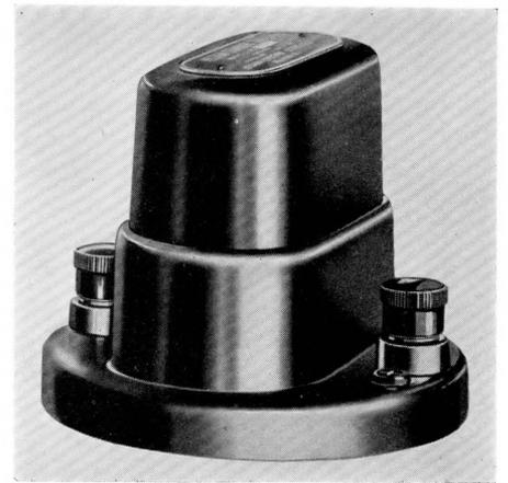
Figure 3—Weston Model 4 Standard Cell
