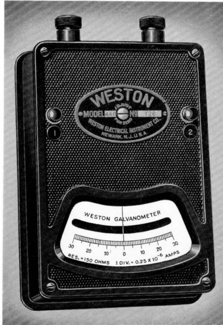
Figure 2—Weston Model 440 Galvanometer
