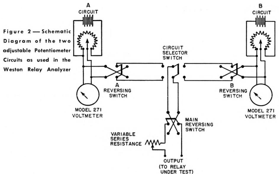
Figure 2—Schematic Diagram of the two adjustable Potentiometer Circuits as used in the Weston Relay Analyzer
