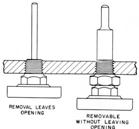
Figure 6—The above sketch illustrates the use of the thermometer with and without its protective socket.
