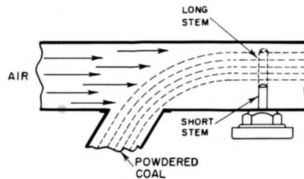
Figure 7—The use of the short stem thermometer is another solution to the erosion problem.
