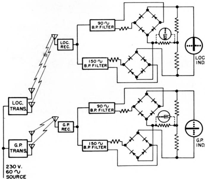
Figure 2—Simplified block diagram of the blind landing transmitting and receiving equipment.
