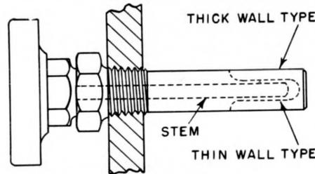
Figure 4—Sketch showing the use of the thermometer with a protective socket.
