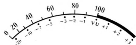
Figure 2—Standard scale for VU Meters.
