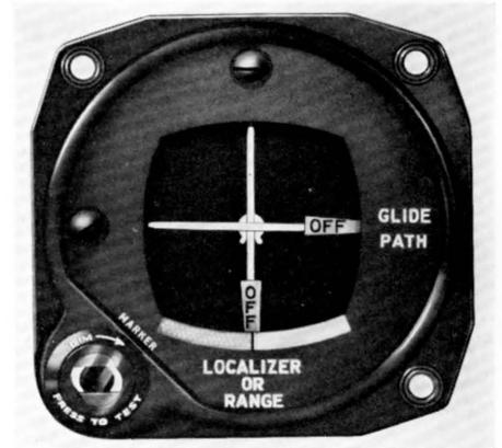
Figure 4—The Weston Model 888 showing inoperative condition of ground or airborne equipment.
