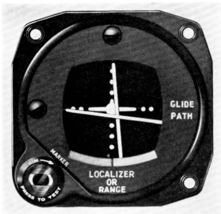
Figure 3—The Weston Model 888 showing operative conditions: ship is slightly above the glide path and slightly left of the localizer course.
