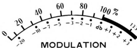
Figure 1—The scale used on FM monitor instruments.
