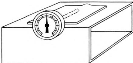
Figure 3—Using the thermometer to indicate surface temperature.
