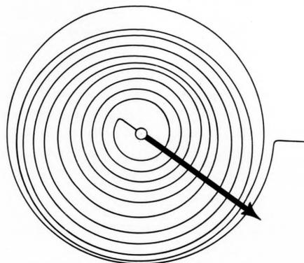
Figure 3b—Note pointer position and shape of coils after a change in temperature. Friction occurs in the turns of the coil and at pointer bearing.
