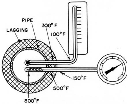
TEMPERATURE GRADIENTS SUCH AS SHOWN MAY CAUSE VARIABLE AND LARGE ERRORS IN GLASS STEM AND OTHER LIQUID OR GAS EXPANSION TYPE THERMOMETERS.
