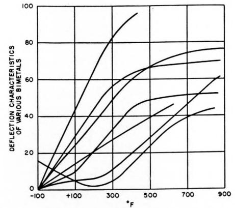
Figure 1—Temperature-deflection characteristics of various bimetals.
