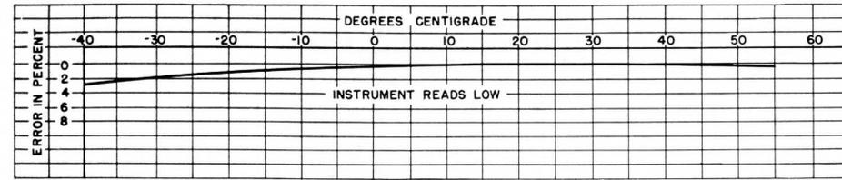
Figure 2—Curve showing temperature compensation of d-c current and voltage ranges.
