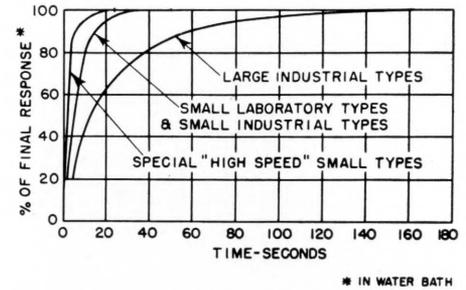
Figure 8—Response time characteristics of various types of Weston thermometers when immersed in liquid.
