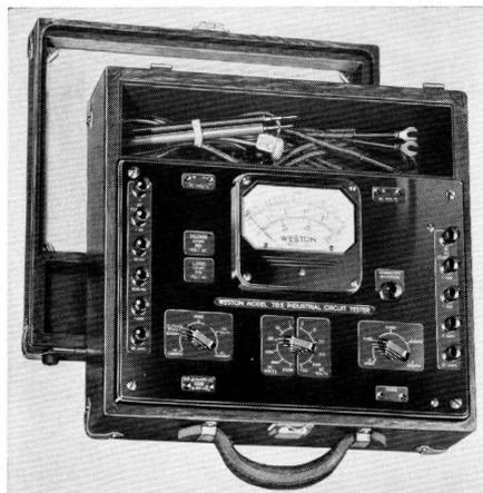
Figure 1—The Weston Model 785, Type 3 Industrial Circuit Tester.
