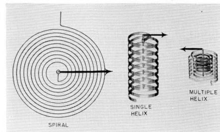
Figure 4—Relative size of three types of bimetal elements having the same torque and deflection.
