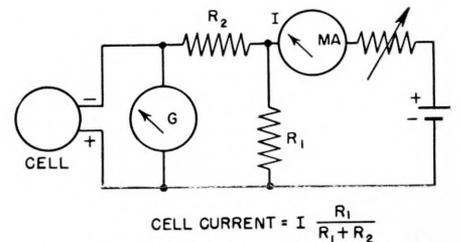
Figure 5—Current balance circuit with attenuator.
