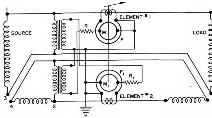
Figure 8—Diagram of connections for a two-element electrodynamic wattmeter for measuring vars in a two phase four-wire circuit.
