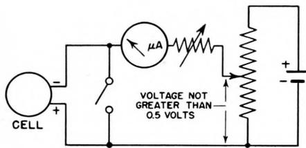
Figure 7—Simplified current balance circuit using a microammeter as the balance indicator.
