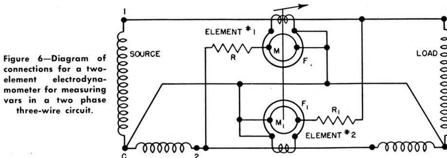
Figure 6—Diagram of connections for a two-element electro-dynamometer for measuring vars in a two phase three-wire circuit.
