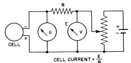
Figure 6—Current balance circuit using a variable voltage source.
