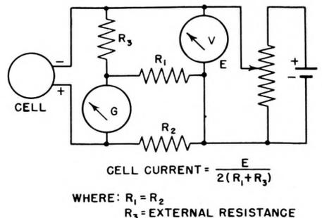
Figure 10—Negative resistance current balance circuit using a variable voltage source.
