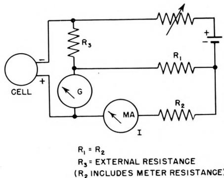
Figure 8—Negative resistance current balance circuit.
