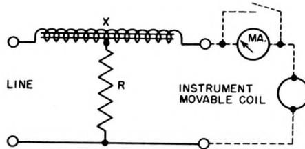
Figure 2—Circuit of reactor for single phase varmeter.
