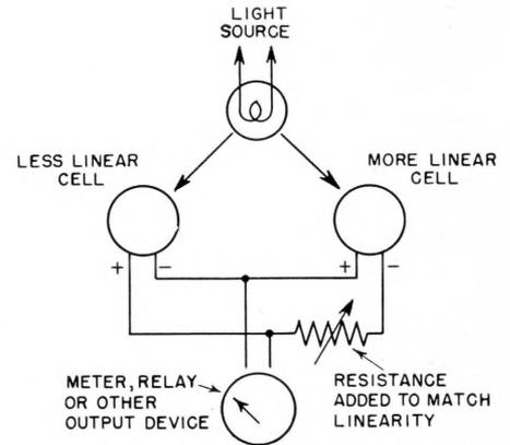
Figure 11—Matched linearity differential circuit.
