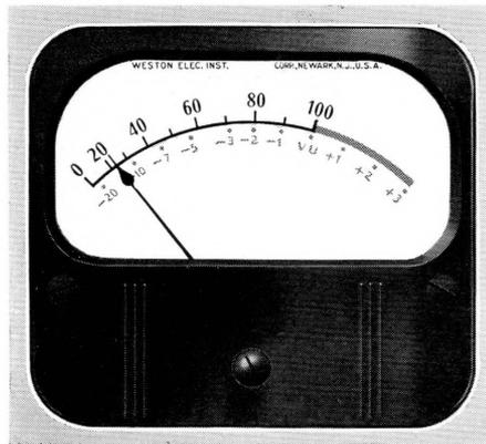
Figure 1—The Weston Model 862, Type 30B VU Meter.
