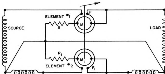
Figure 5—Diagram of connections for a two-element electro-dynamometer for measuring vars in a two phase three-wire circuit.
