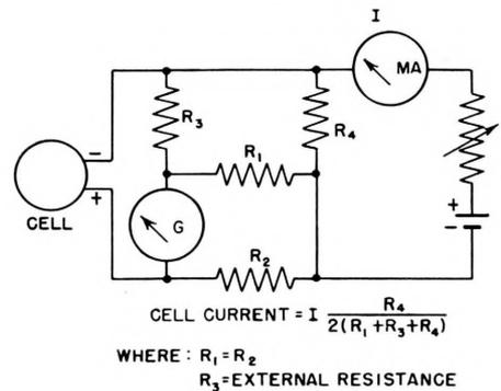
Figure 9—Negative resistance current balance circuit with attenuator.
