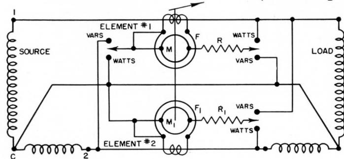
Figure 7—Diagram of connections for a two-element electrodynamic wattmeter for measuring watts or vars in a two phase three-wire circuit.
