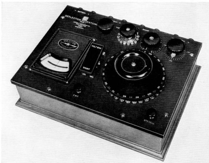
Figure 4—Leeds and Northrup Model 7 Brooks Deflection Potentiometer.
