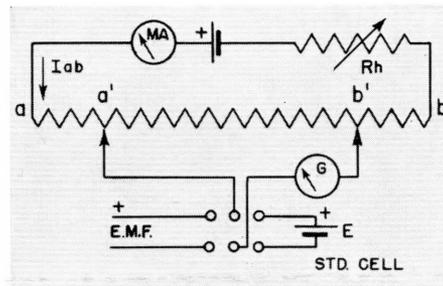
Figure 2—Diagram of a simplified potentiometer circuit.
