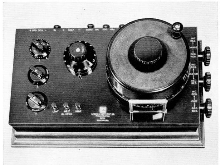
are made so that even values of potential can be read directly. Figure 3 shows a Leeds and Northrup Type K-2 precision potentiometer.
