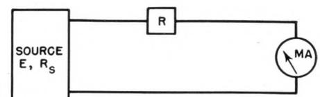
Figure 1—Circuit for determining the resistance of a power source by resistance-doubling method.
