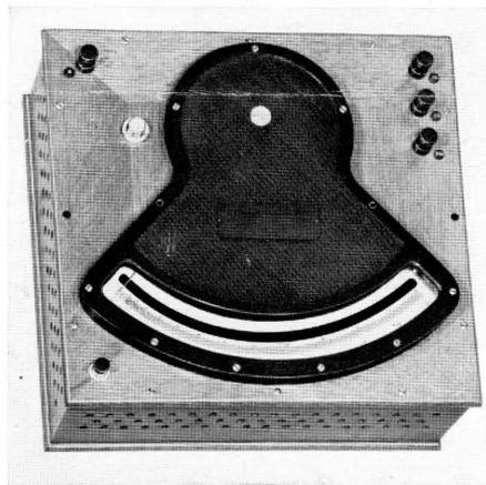
Figure 5—The Weston Model 326 Voltmeter.
