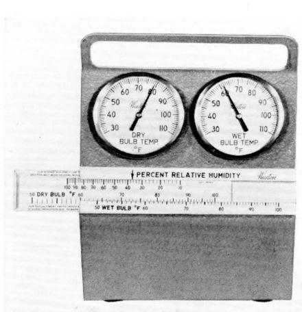
Figure 2—Front view of Humidity Indicator illustrating use of the slide rule calculator.
