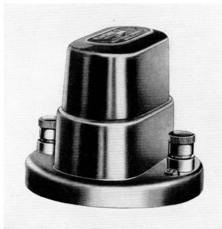
Figure 1—The Weston Model 4 Standard Cell.
