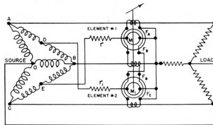
Figure 22—Schematic connections for a two and one-half element varmeter to a three-phase four-wire system using current transformers and a phase shifting reactor.
