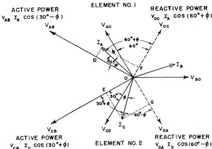
This method and basic instrument may be used to measure reactive power directly by selecting or constructing potentials displaced by 90 degrees from the potentials used to measure the active power.
