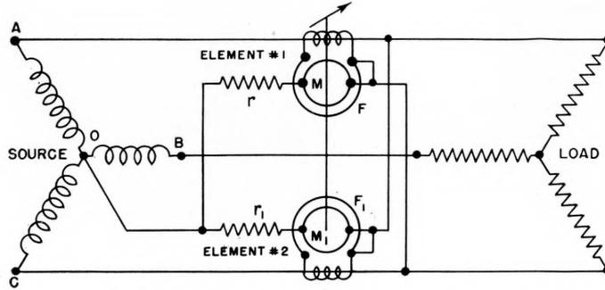
Figure 12—Schematic connections for a two-element wattmeter to a three-phase three-wire system when the neutral is available. Current transformers are used.
