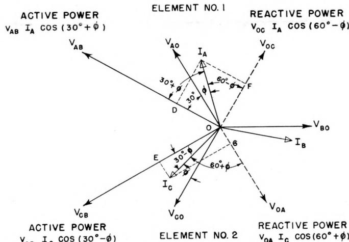
Figure 10—Angular relation between currents and potentials in a three-phase system, when currents lead potentials.
