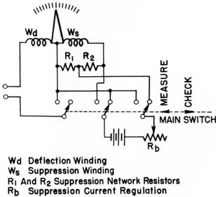
Figure 2—Schematic diagram for electrical zero suppression.
