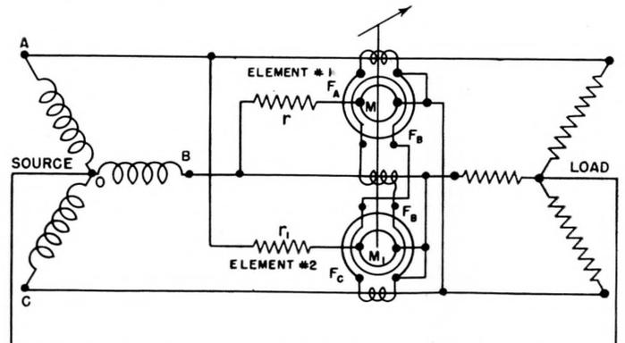
Figure 21—Schematic connections for a two and one-half element varmeter to a three-phase four-wire system using current transformers.
