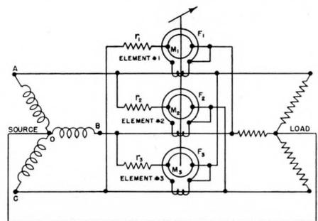
Figure 24—Schematic connections for a three-element varmeter to a three-phase four-wire system using current transformers.
