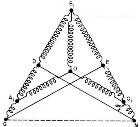
Figure 16—Relation of potentials in a phase shifting reactor for use on three-phase three-wire systems.
