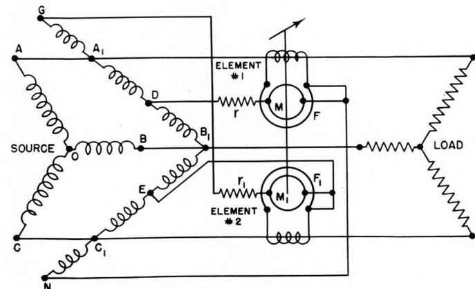
Figure 15—Schematic connections for a two-element varmeter to a three-phase three-wire system using a phase shifting reactor and current transformers.
