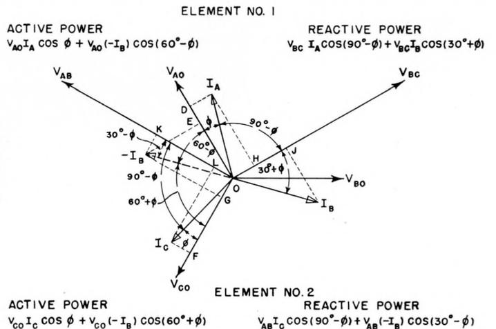
Figure 20—Angular relation between currents and potentials in a three-phase four-wire system when currents lag potentials.
