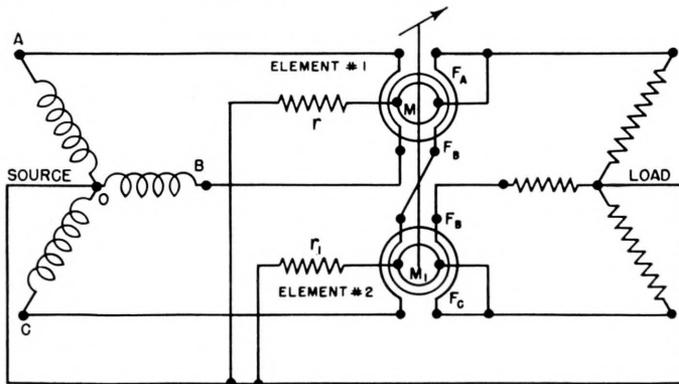
Figure 19—Schematic connections for a two and one-half element wattmeter to a three-phase, four-wire system.
