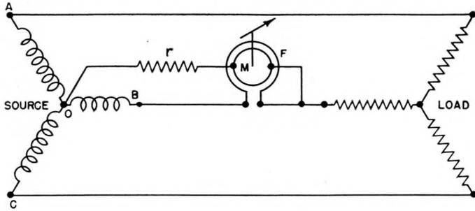
Figure 17—Schematic connections for a single-element wattmeter to a balanced three-phase three-wire system.
