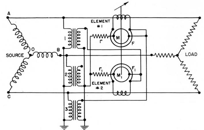
Figure 14—Schematic connections for a two-element varmeter to a three-phase three-wire system using potential and current transformers.
