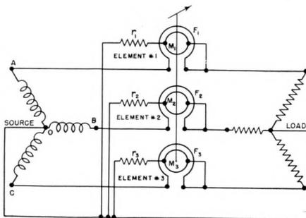
Figure 23—Schematic connections for a three-element wattmeter to a three-phase four-wire system.
