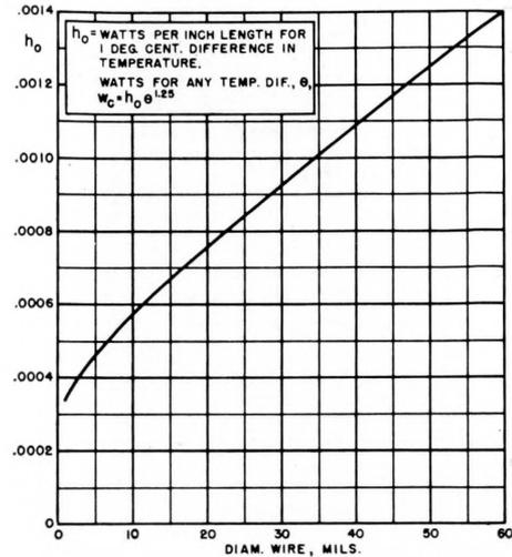
**Figure 8. Convection coefficient  $h$  for single wires mounted horizontally in still air, in watts per inch length for 1 deg. cent. difference in temperature. Watts loss for any temperature difference  $\theta$ , is  $W_o = h_o \theta^{1.25}$ .**
