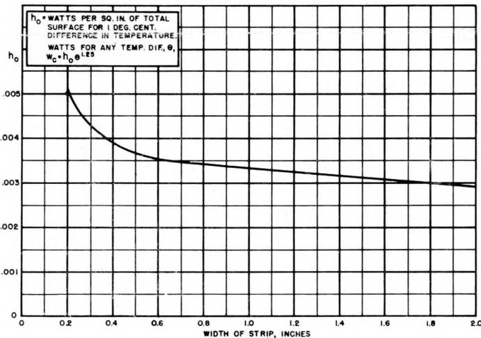
**Figure 7. Convection coefficient,  $h_o$ , for a single strip mounted horizontally with its surfaces vertical, or for a relatively large diameter tube with its axes vertical, in still air, in watts per sq. in. for 1 deg. cent. difference in temperature. Watts loss for any temperature difference  $\theta$ , is  $W_o = h_o \theta^{1.25}$ .**
