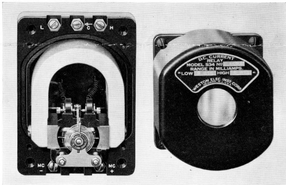
Normal Pressure Type Relay with cover removed—Weston Model 534
