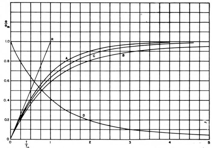
CURVE A. Temperature change of the body with time when heat is added from an external source at a constant rate.
