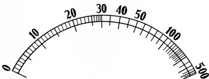
Figure 4—A typical scale showing expanded and contracted divisions.
