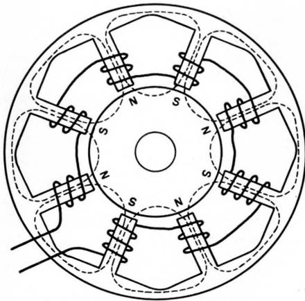
Figure 6—A stator assembly used for charging the magnet.
