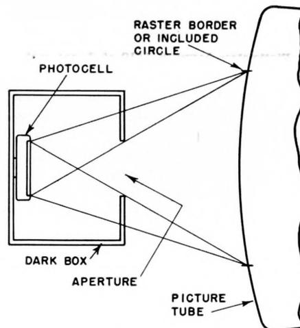
Figure 1—A suggested sighting arrangement with aperture.
