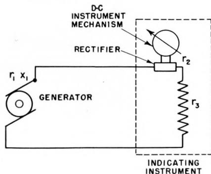
Figure 7—A typical circuit diagram for the a-c generator and indicator.
