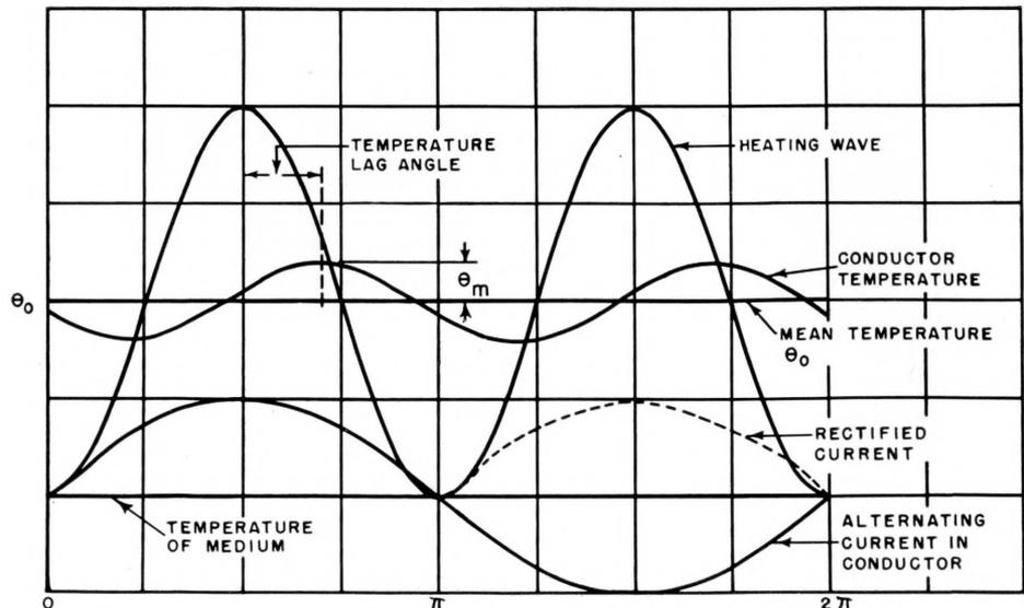
Figure 12—Temperature pulsation in a conductor heated by alternating current or full wave rectified current.
