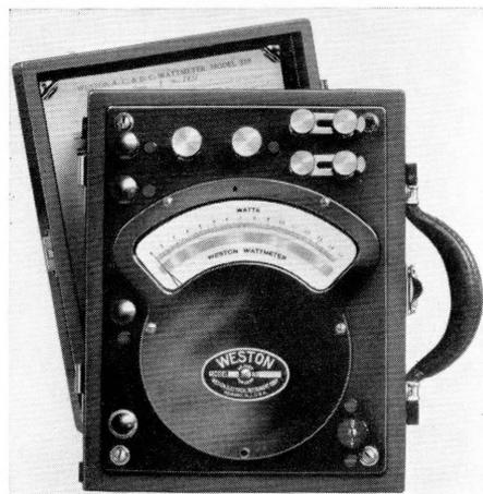
Figure 1—Weston Model 310 Single Phase Wattmeter—Accuracy  $\frac{1}{4}$  of 1 per cent.
