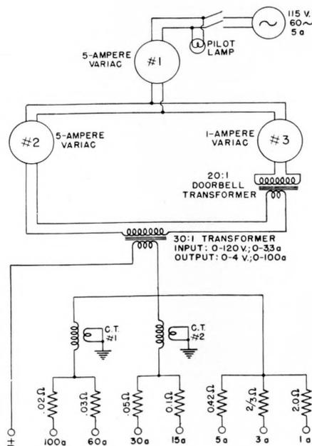
Figure 1—Circuit for current calibrations.
