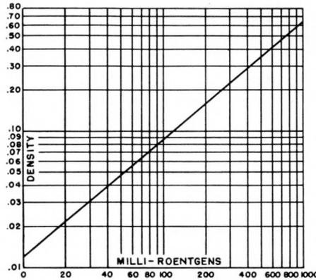
Figure 4—A typical calibrated curve of Milli-roentgens Exposure against Density.
