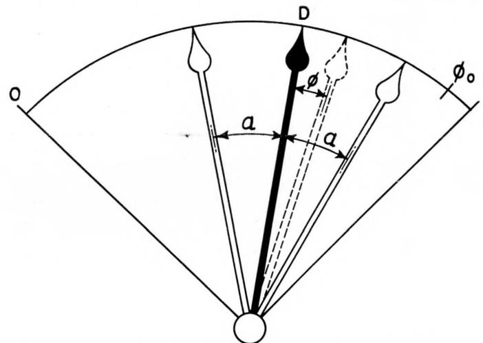
Figure 13—Oscillation of an instrument pointer resulting from the alternating or pulsating torque produced by alternating or rectified current, and specifically by the pulsating current generated in a thermocouple connected to a conductor carrying alternating current which produces cyclic pulsations in temperature.
