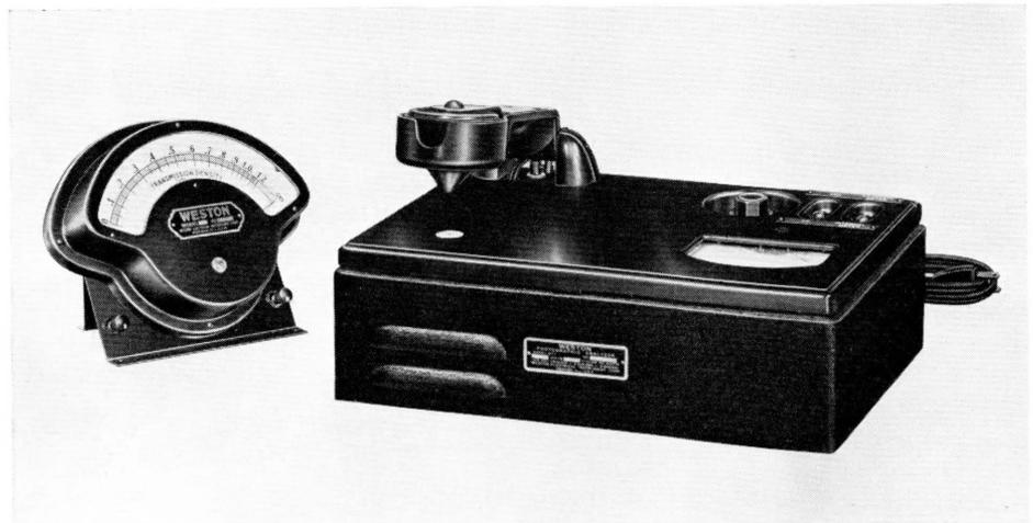
Figure 5—The Weston Model 877, Type 5 Health Protection Densitometer and its auxiliary long-scale meter.
