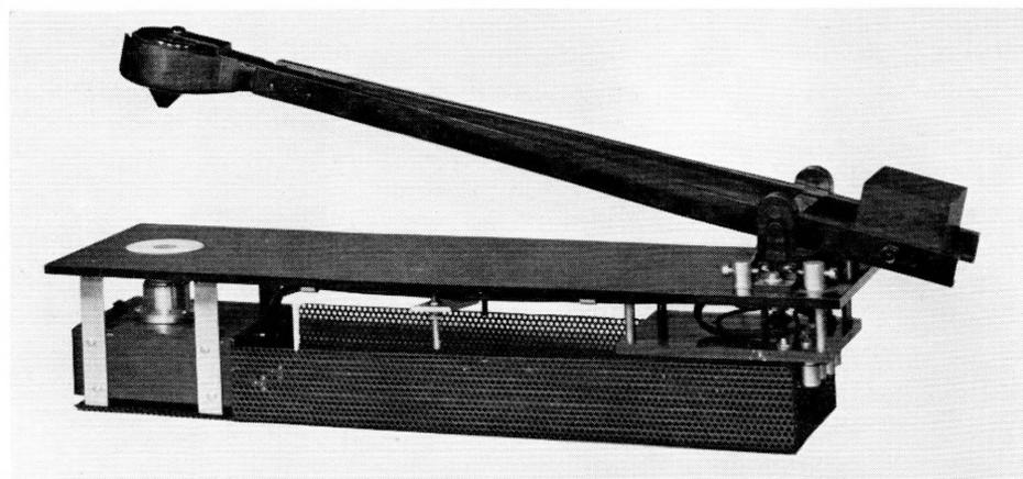
Figure 3—The Weston Model 870 Densitometer is designed to accommodate photographic plates as large as 30 x 40 inches.
