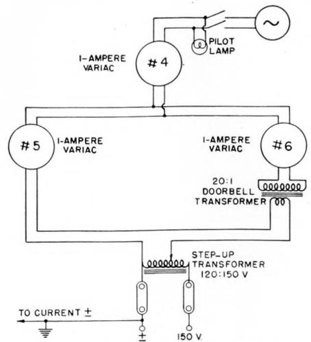
Figure 2—Circuit for potential calibrations.
