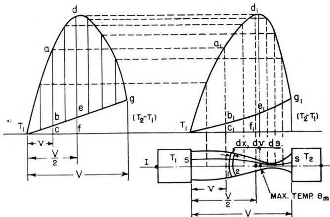
Figure 14—Steady state temperature distribution along a conductor of any shape connected between terminals having unequal temperatures, when the conductor is heated by an electric current passing through it, and all the heat generated is dissipated by conduction to the terminals.
