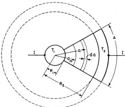
Figure 16—Location of the maximum temperature in a circular disc or a sector thereof, having a circular terminal at its center, and a ring terminal at its rim, when heated by a current passing through the disc between terminals. Maximum temperature lies at a radius  $a_m = \sqrt{R_1 R_2}$ .
