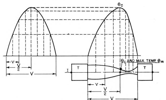
Figure 15—Steady state temperature distribution along a conductor of any shape connected between terminals having equal temperatures, when the conductor is heated by an electric current passing through it, and all the heat generated is dissipated by conduction to the terminals.
