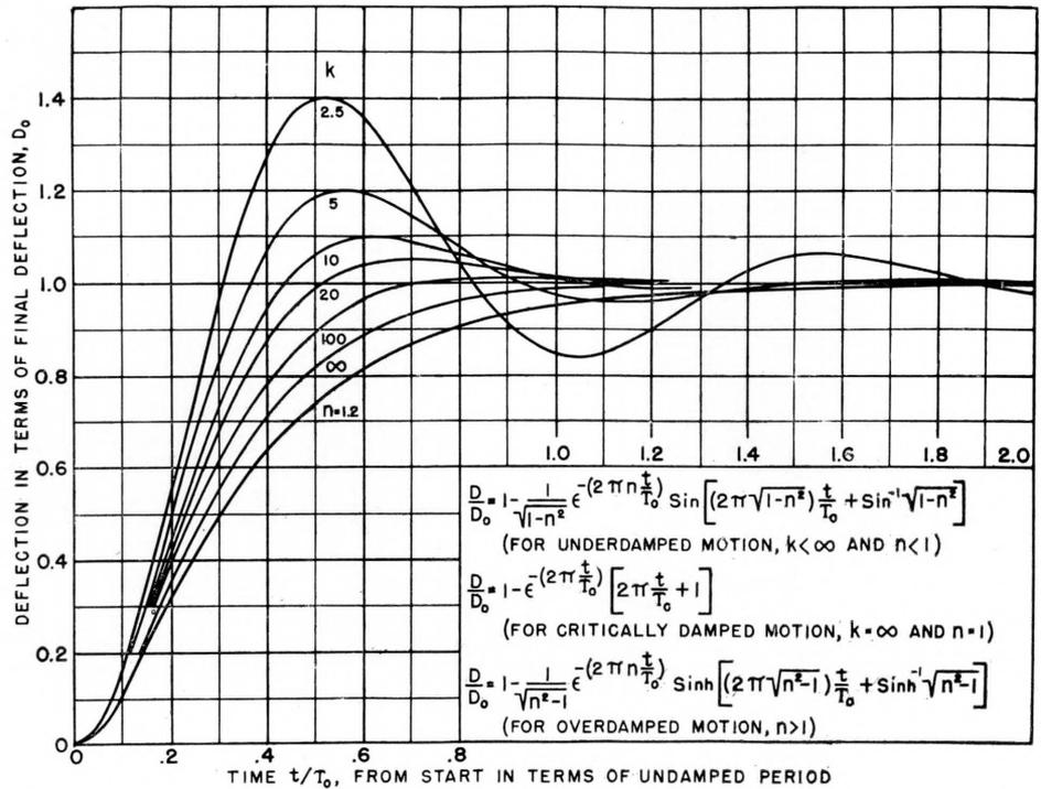
Curves of damped periodic motion of an instrument pointer for any value of undamped period,  $T_0$ .
