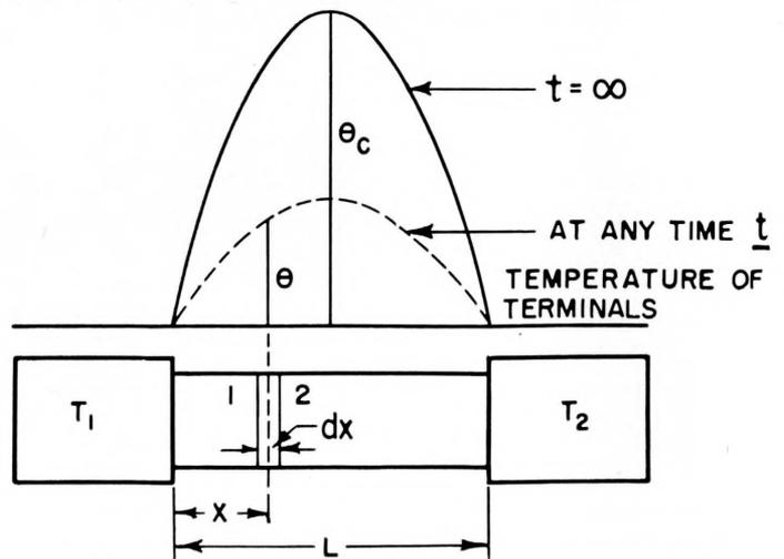
Figure 17—Temperature-time distribution diagram for a conductor connected between heat absorbing terminals, heated uniformly at a constant rate and, in general, cooled by conduction to the terminals, and by convection to the surrounding medium.
