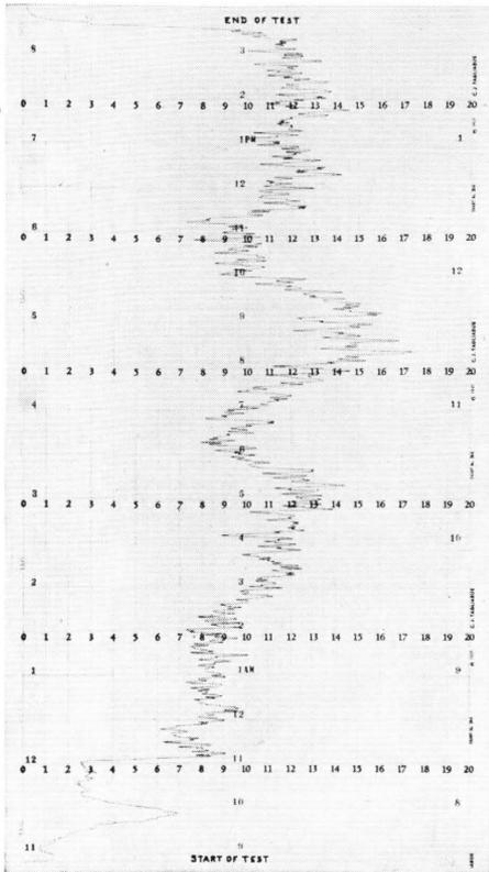
Figure 1—A reduced copy of an actual record made on a ten-minute type of red fusee.
