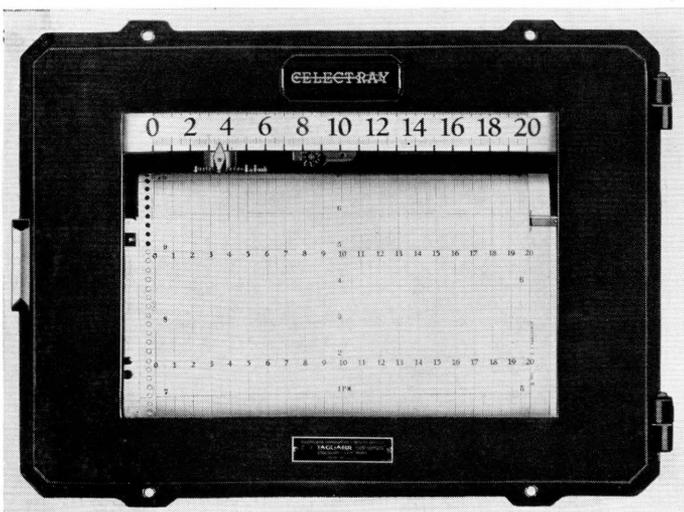
Figure 2—The TAG CELECTRAY Recorder illustrated here is a photo-mechanical type in which a mirror type of galvanometer reflects light on and off a phototube.
