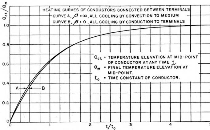
Figure 18—Temperature-time heating curves for the mid-point of the heated general conductor, as illustrated and described in Figure 17, for various values of thermal length,  $\beta$ . To make the curves universally applicable, temperatures are given relative to the maximum temperature  $\theta_m$ , and time, relative to the time constant,  $t_0$ . Note: The curves for  $\beta=8$ , and  $\beta=0$  are so nearly alike that they are difficult to separate in drawing.
