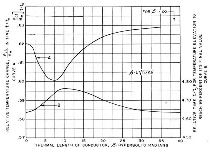
Figure 19—Temperature-time relations in a heated general conductor, as illustrated in Figure 17. Curve A shows the increase in temperature,  $\theta_{ct}$ , at the mid-point, relative to the maximum temperature,  $\theta_m$ , which takes place in a time equal to the time constant  $t_0$ . Curve B shows the time, relative to the time constant  $t_0$ , required for the temperature increase to reach 99 per cent of its final value  $\theta_m$ , both for various values of thermal length,  $\beta$ .
