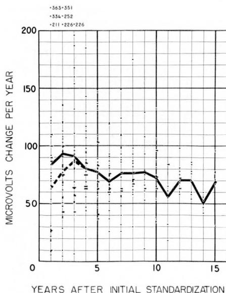
Figure 1—Graph showing voltage drift of standard cells with age.
