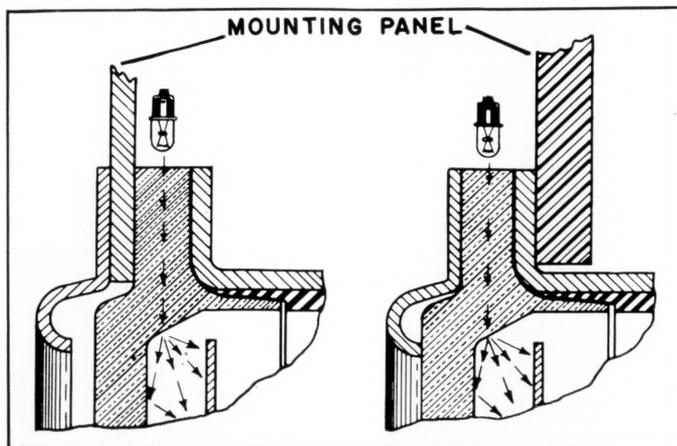
Figure 5—Details of edge lighting means showing the relative position of mounting panel.
