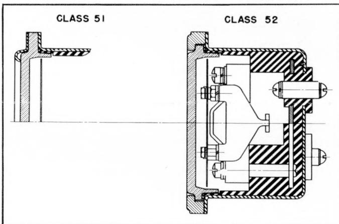
Figure 1—Sectional view of 2½" and 3½" d-c instruments. Class 51 is shown for comparison.
