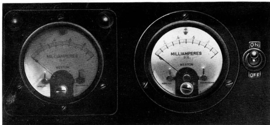
Figure 6—The above illustration shows the comparison of a non-illuminated and edge-lighted dial.
