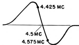
Figure 11—Properly adjusted sound IF and discriminator.
