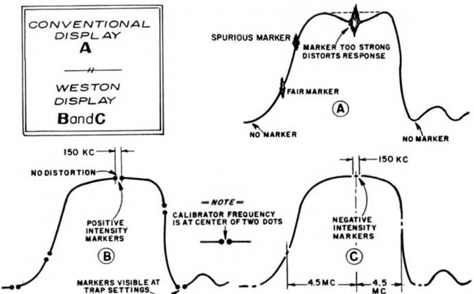
Figure 16—Weston intensity marker display vs conventional marker pip display.
