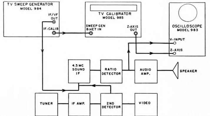
Figure 22—Weston Simplified Method of checking over-all sound IF response and discriminator characteristics of intercarrier systems.
