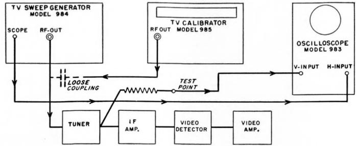
Figure 15—Conventional method of checking tuner response.
