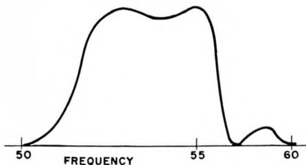
Figure 4—Response of receiver to unit voltage variable frequency signal.
