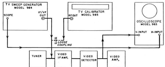
Figure 13—Conventional method of checking video IF response.
