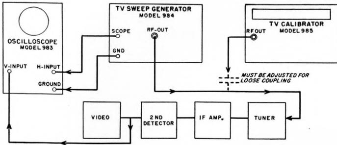
Figure 14—Conventional method of checking over-all response characteristics.
