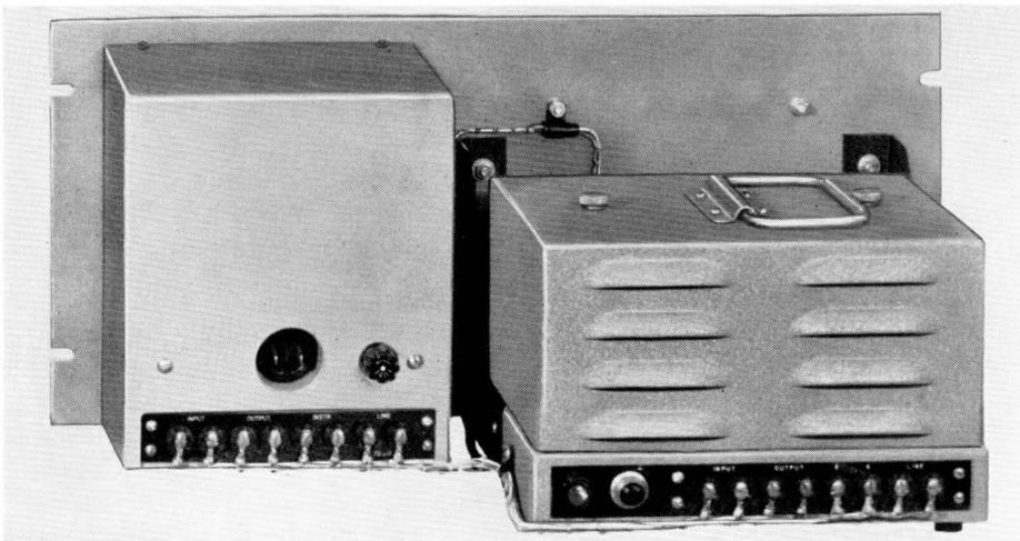
Figure 2—Rear panel layout of the Model 1411 Amplifier and rectangular metal box enclosing the range network as a unit.
