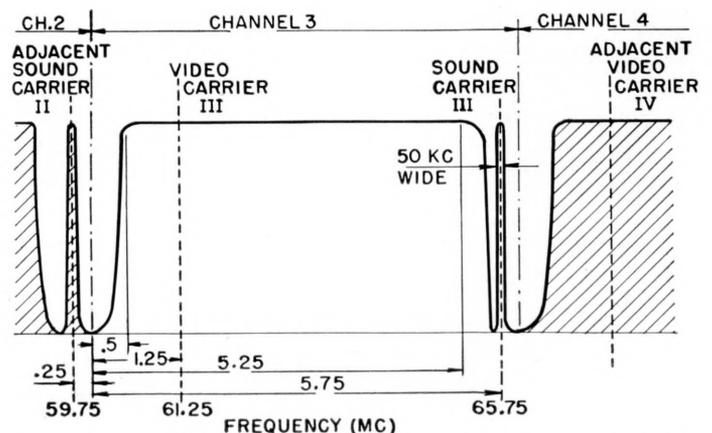
Figure 1—Frequency allocation of Channel 3, together with adjacent Channels 2 and 4.
