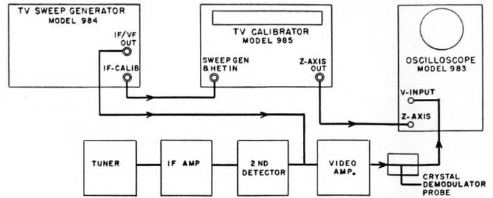
Figure 21—Weston Simplified Method of checking video amplifier response.
