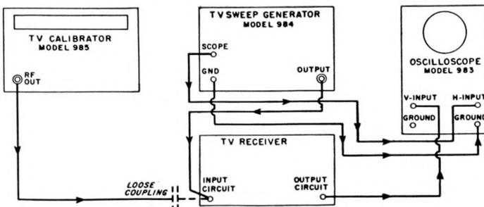
Figure 12—Television alignment procedure (Method 1).
