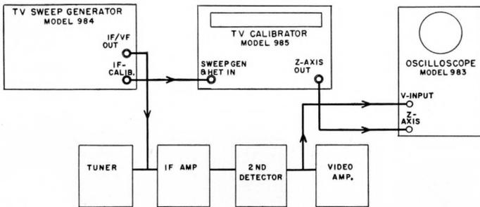
Figure 19—Weston Simplified Method of checking video IF response characteristics.
