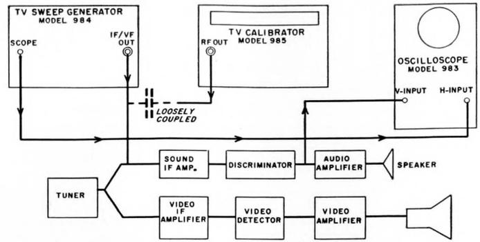
Figure 3—Conventional method of checking over-all sound IF response and discriminator characteristics of Split Sound System.
