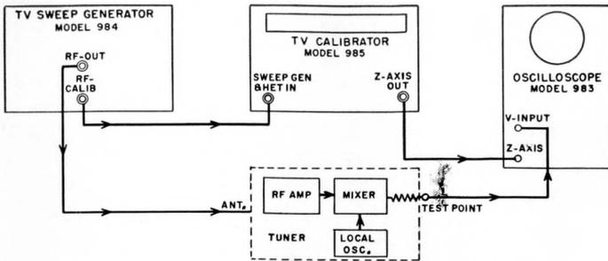
Figure 18—Weston Simplified Method of checking tuner response.
