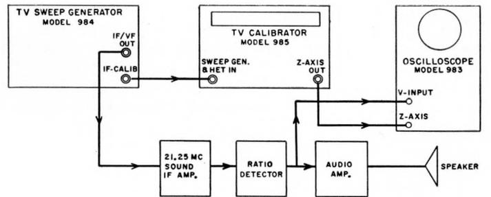
Figure 23—Weston Simplified Method of checking over-all sound IF response and discriminator characteristics of split carrier systems.
