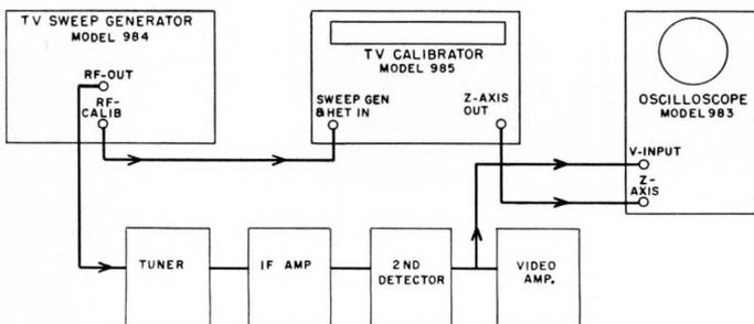
Figure 20—Weston Simplified Method of checking over-all response.
