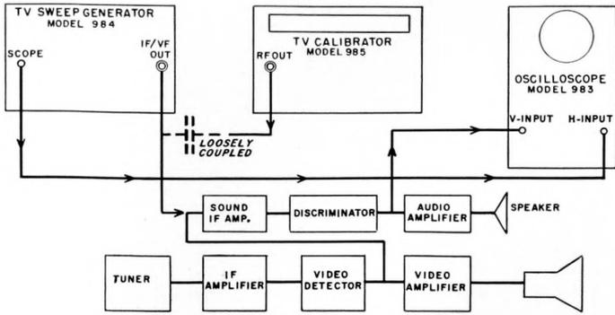
Figure 2—Conventional method of checking over-all sound IF response and discriminator characteristics of intercarrier systems.
