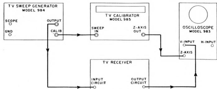
Figure 17—Weston Simplified Method of alignment (Method 2).
