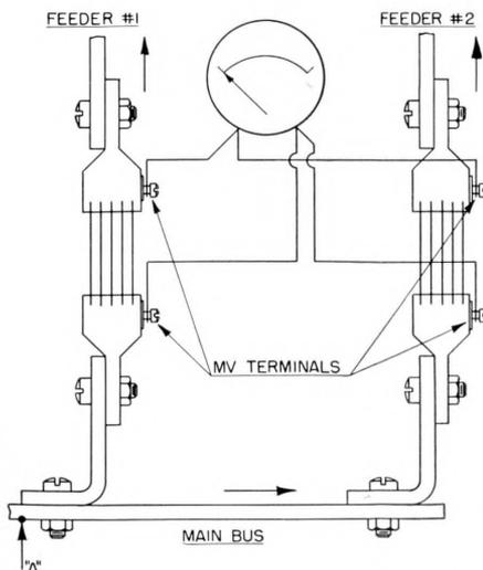
Figure 1—Two individual shunts connected in two bus bar feeders.
