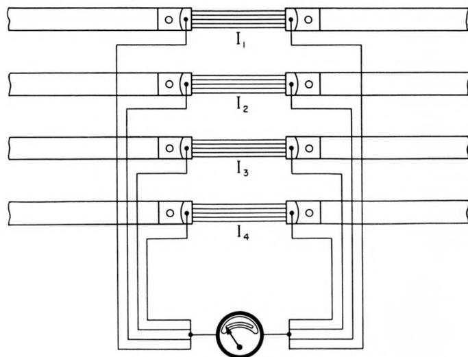
Figure 5—One method for connecting shunts in parallel.
