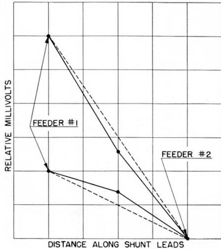
Figure 4—No current in feeder No. 2; original current in feeder No. 1.
