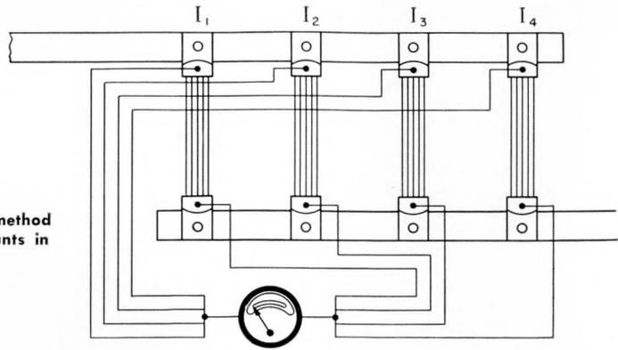
Figure 6—Another method for connecting shunts in parallel.
