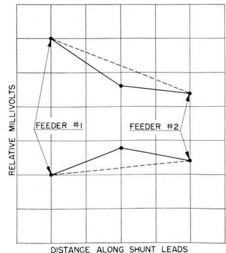
Figure 3—Current in feeder No. 2 reduced by half; original current in feeder No. 1.
