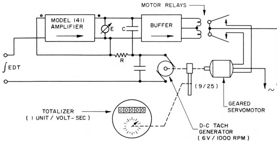
Figure 1—Block diagram of Model 1473 Precision Integrator.
