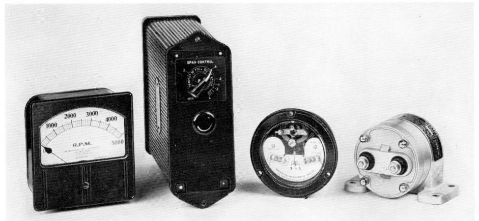
Figure 1—The Component Parts of the Automatic Speed-Change Sensing System Dismounted From Panel.
