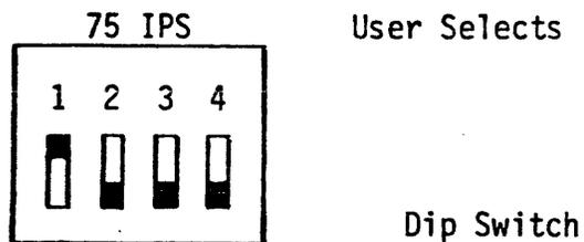
1. Only 1 switch in the UP position at one time.
