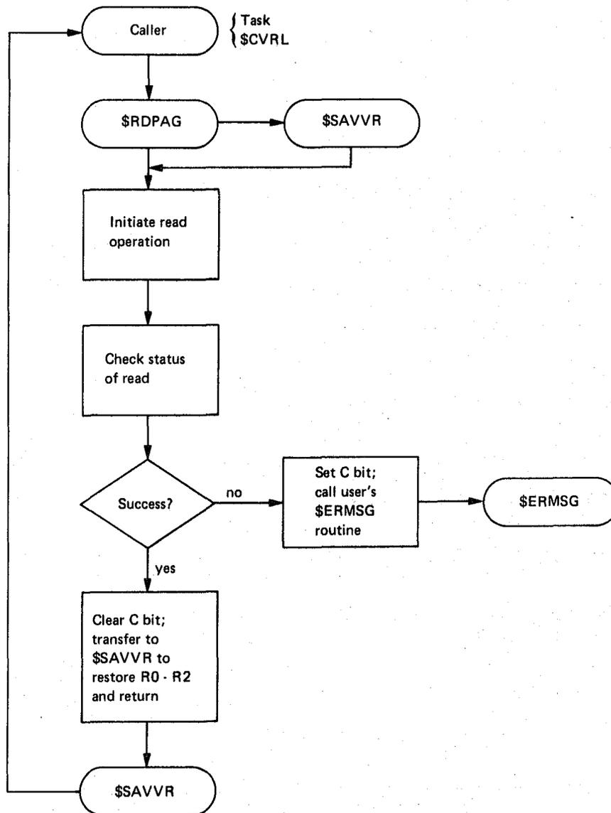
Figure 8-11 General Block Diagram of the \$RDPAG Routine
