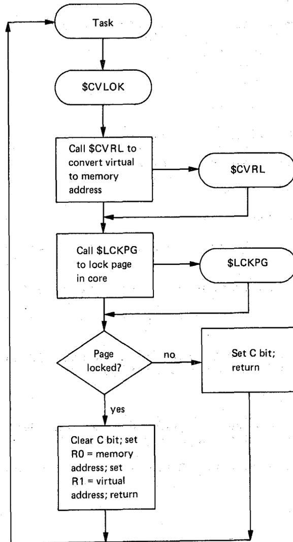
Figure 8-9 General Block Diagram of the \$CVLOK Routine
