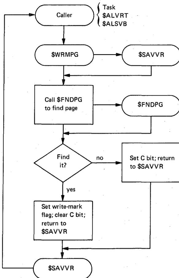
Figure 8-13 General Block Diagram of the \$WRMPG Routine
