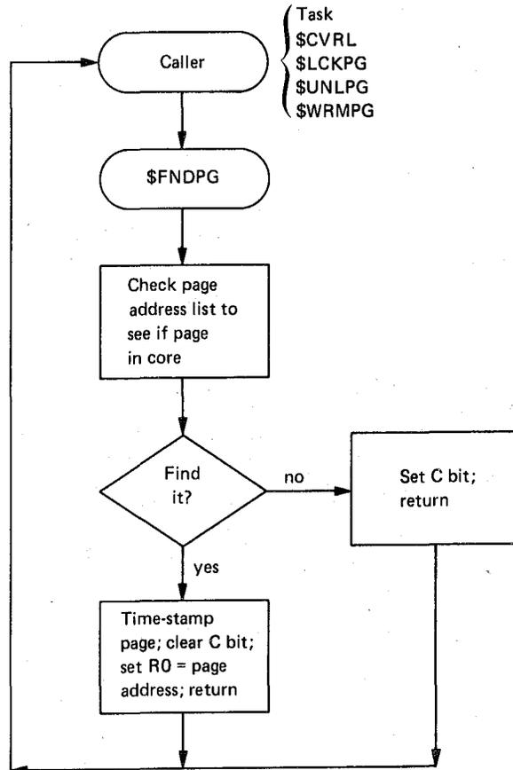
Figure 8-12 General Block Diagram of the \$FNDPG Routine
