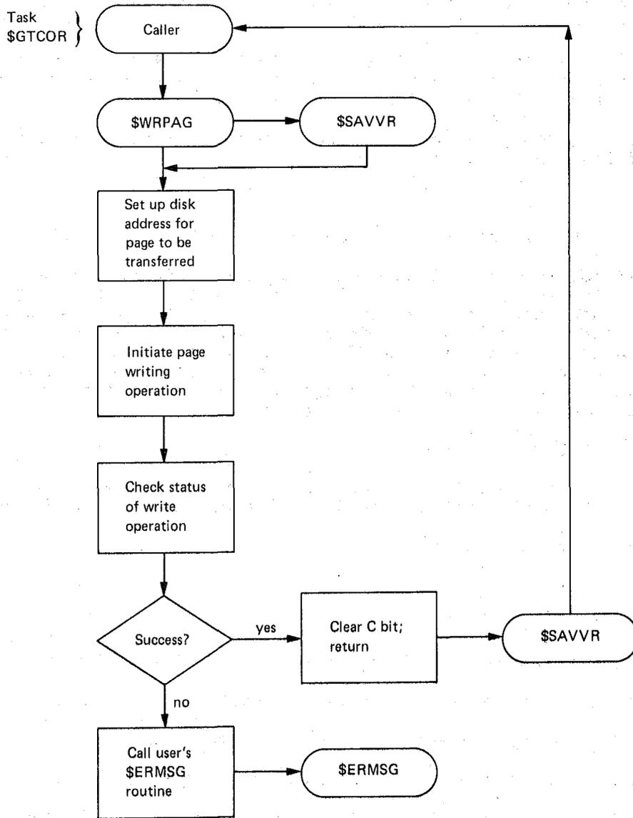
Figure 8-5 General Block Diagram of the \$WRPAG Routine
