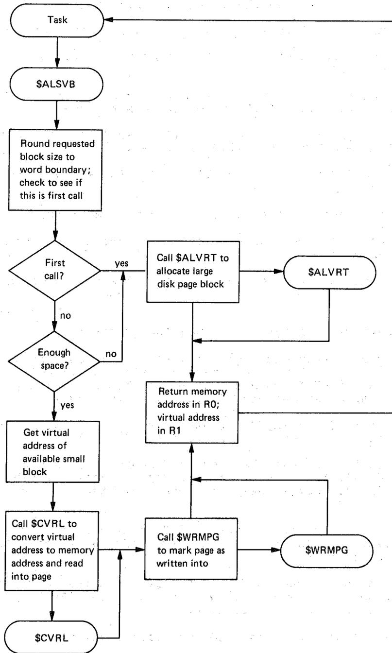
Figure 8-7 General Block Diagram of the \$ALSVB Routine
