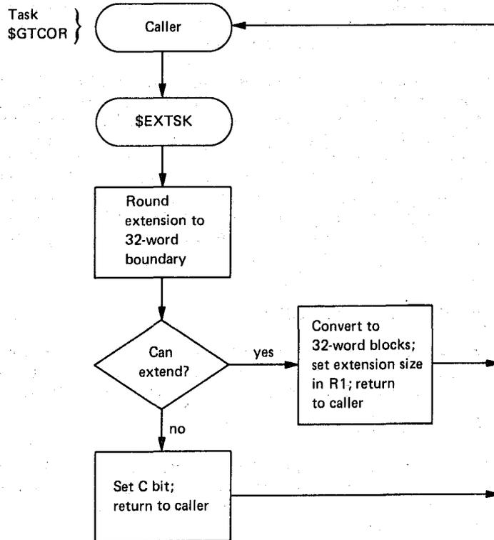
Figure 8-4 General Block Diagram of the \$EXTSK Routine
