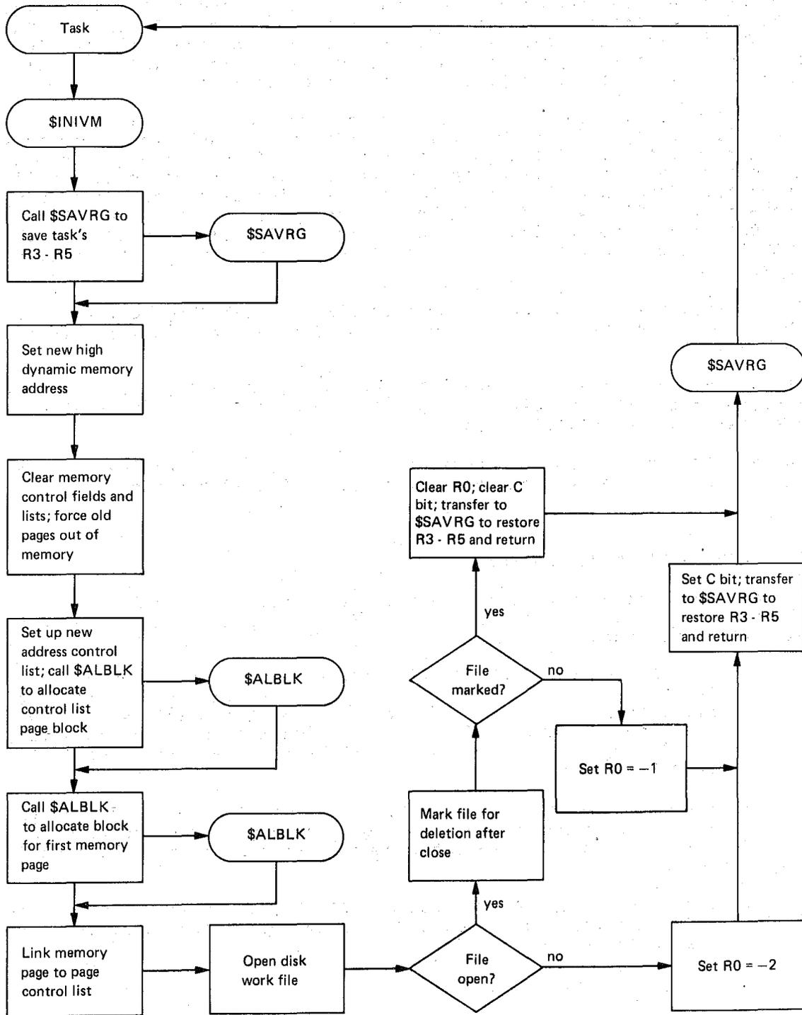
Figure 8-1 General Block Diagram of the \$INIVM Routine
