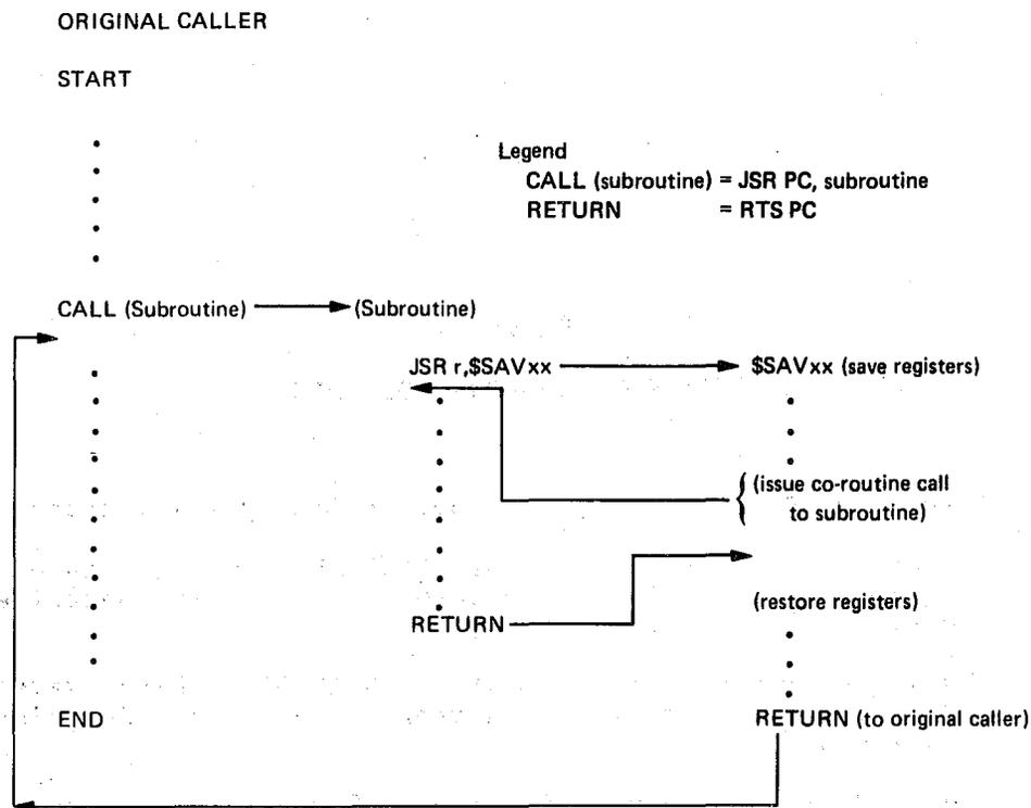
Figure 2-1 Control Swapping of the Register Handling Routines
