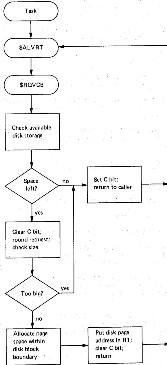
Figure 8-8 General Block Diagram of the \$RQVCB Routine
