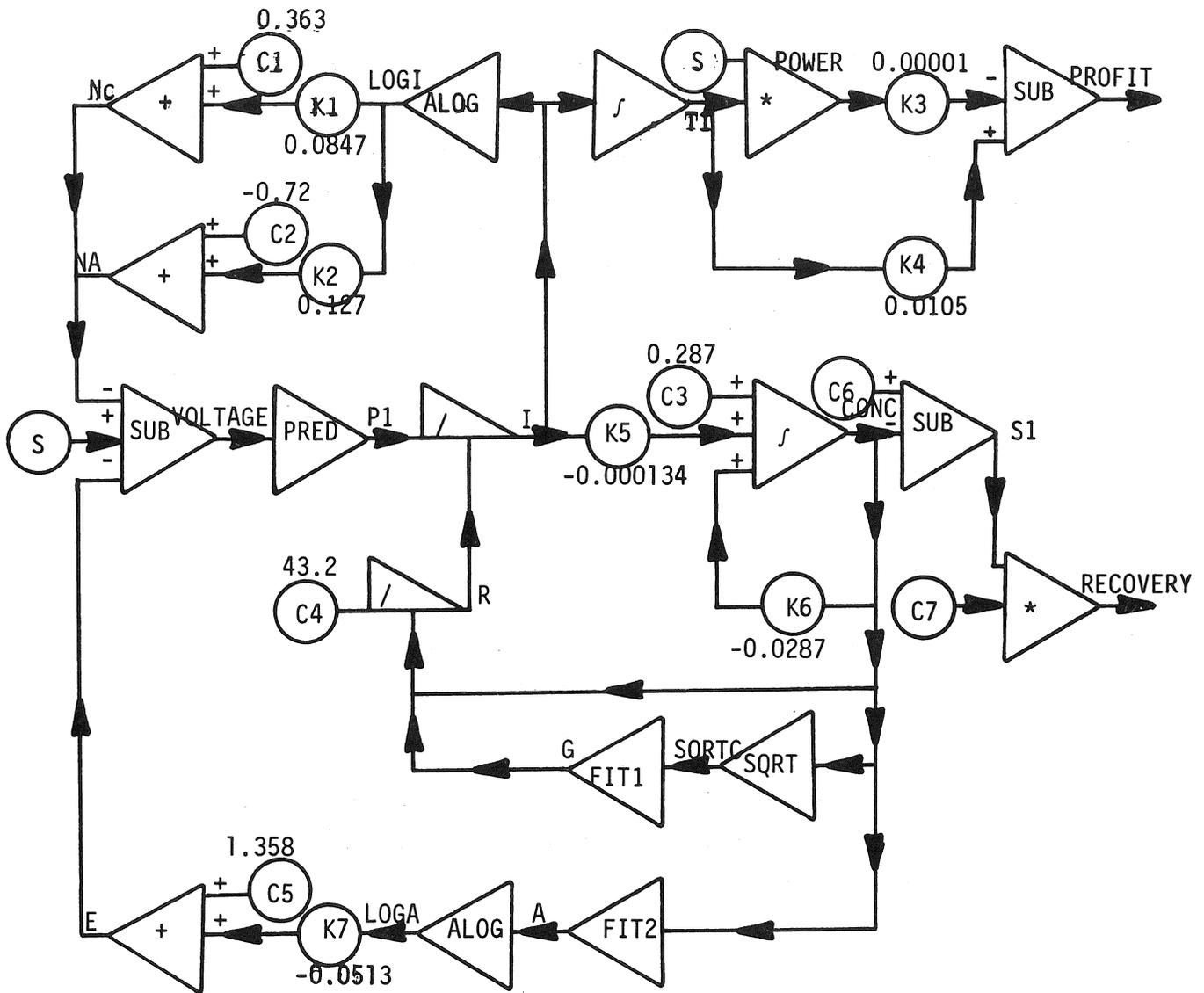
Figure 1. Flowchart for Recovery of Chlorine
