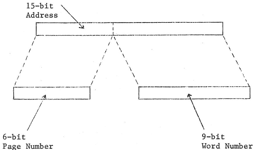
Figure 3 Subdivision of a 15-bit Memory Address
