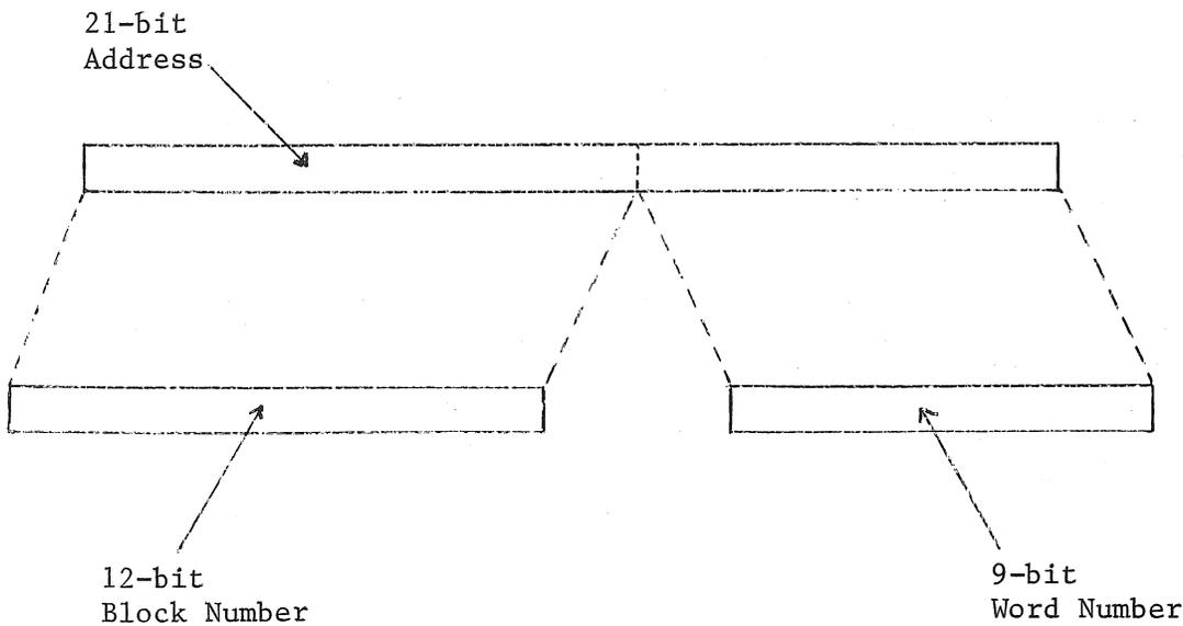
Figure 2 Subdivision of a 21-bit Logical Address
