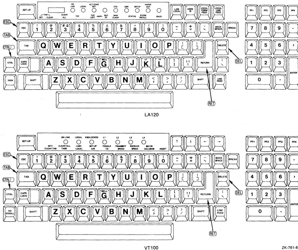
Figure 1-3: The LA120 and VT100 Keyboard Layouts
