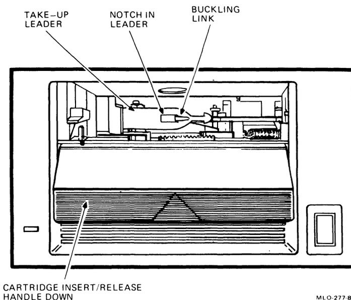
**If the leader is unhooked or if you cannot clearly see the pointed end, DO NOT INSERT THE CARTRIDGE INTO THE DRIVE. DO NOT ATTEMPT TO FIX THE LEADER. Contact your service representative.**
