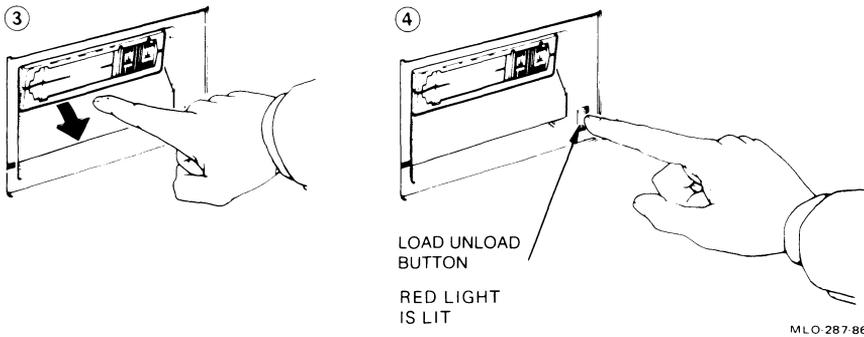
5. The tape loads in 10-15 seconds. During loading the two leaders couple and the tape winds onto the take-up reel inside the tape drive.
