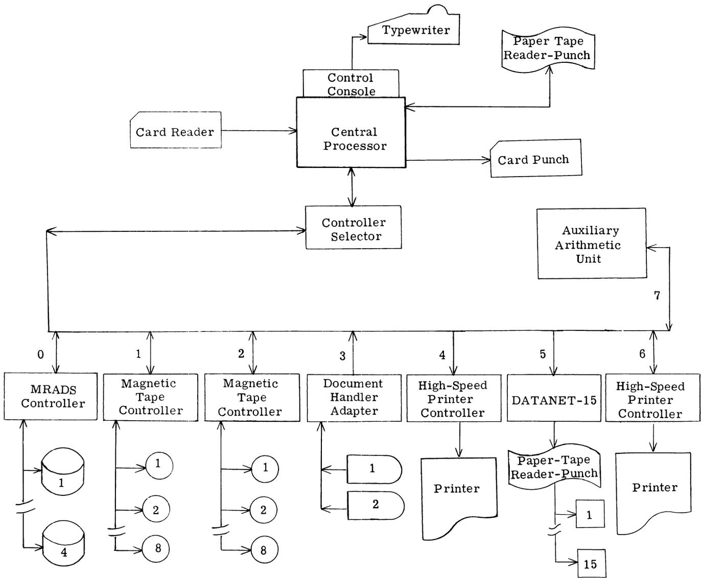
Figure 1-4. Large GE-225 System Configuration
