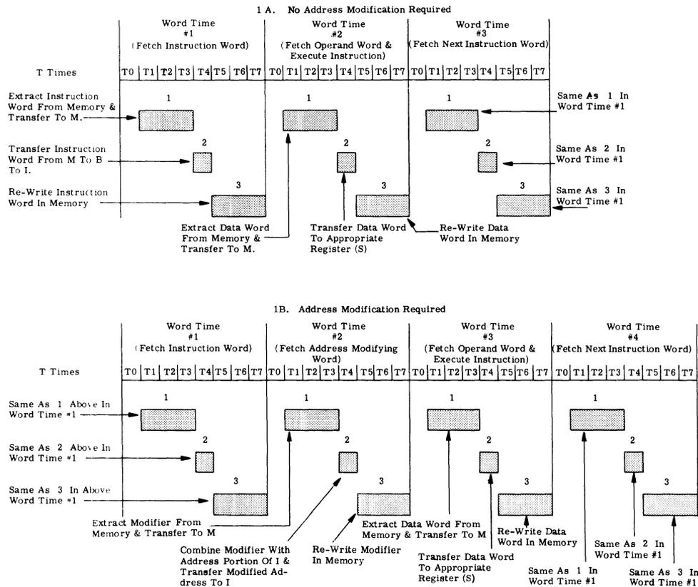
Figure 3-6. Basic Timing for Single Length Word Operations
