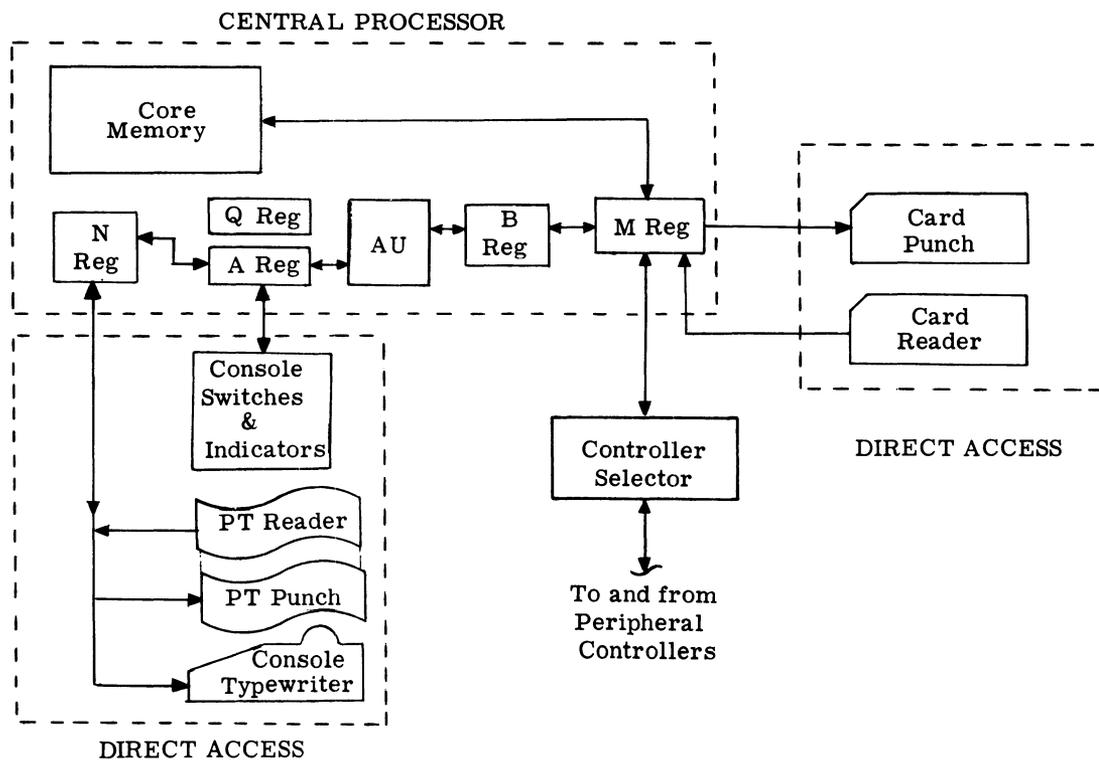
Figure 6-1. Units Directly Accessing Memory
