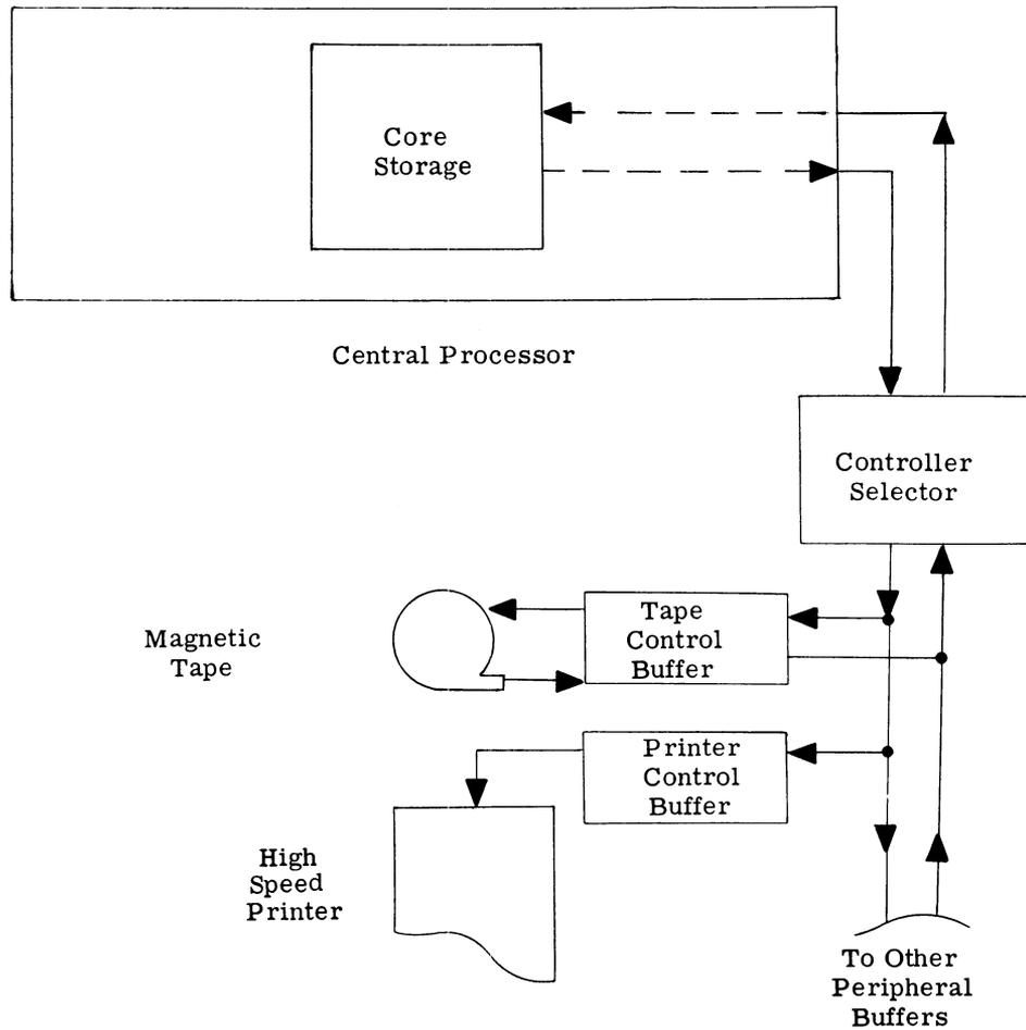
Figure 1-2. Central Processor and Controller Buffers
