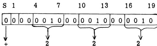
Bit positions 4 through 7, 10 through 13, and 16 through 19 are used to express decimal digits in standard BCD format. Decimal quantities greater than 999 are expressed by using two or more 20-bit words.
