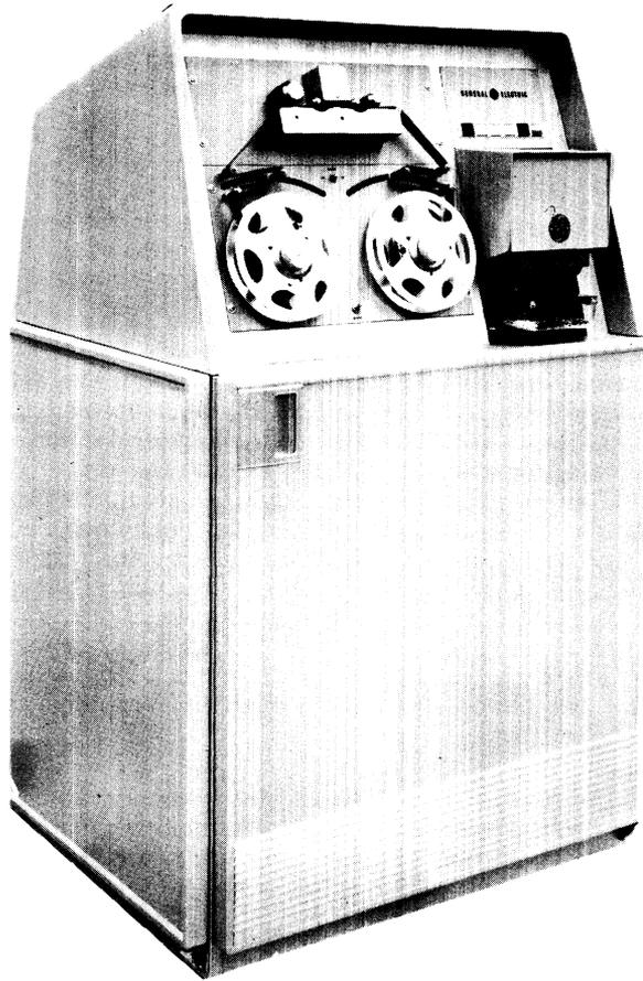
tapes at 250 or 1000 characters per second, and a mechanism for punching five-, six-, seven-, and eight-channel paper tapes at 110 characters per second. Provisions are made to accommodate all common paper tape codes.
