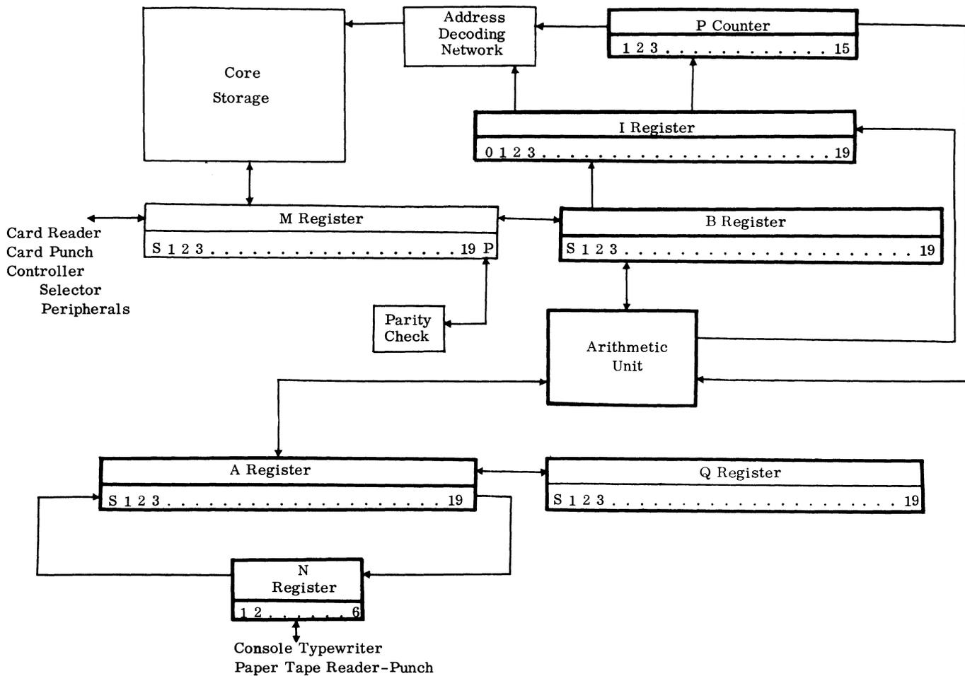
Figure 3-3. GE-225 Arithmetic and Control Register
