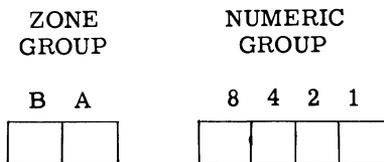
The numeric bits correspond to the first four powers of two, as they do in the binary system, and can express up to 16 numeric values, 0 through 15. The zone bits provide for coding alphabetic and special characters.
