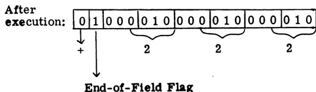
**Comments:** The OCT 1000000 places the flag constant in storage; LDA MILL and ORY DECW insert a 1-bit into bit position 1 of DECW (the high-order word).
