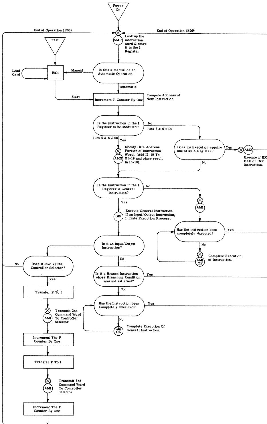
Figure 3 - 8: Flow Chart Showing Central Processor Operating Cycle
