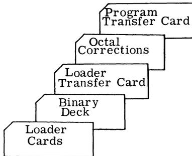
The octal corrections are punched as follows: One card is punched for each change to be made. Columns 5 through 9 contain the octal address and columns 12 through 18 contain the octal contents required. Figure 13-14 shows a sample octal correction card.
