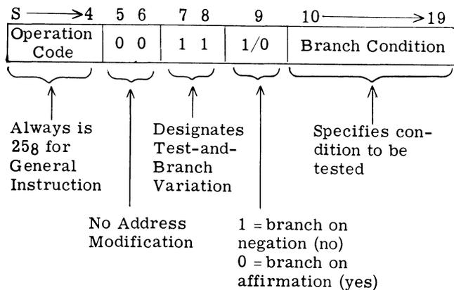
The specific bit patterns for all Format II instructions can be found by converting the octal equivalent of the instructions to binary. The octal form of each instruction is included in the instruction descriptions in subsequent sections.
