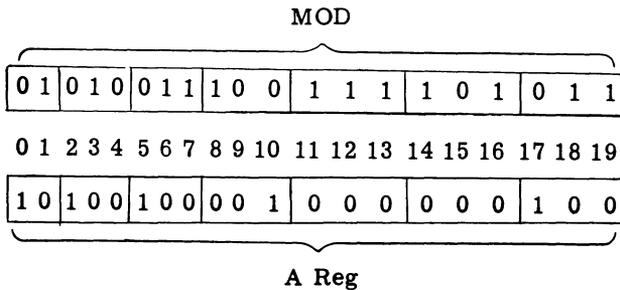
**Example 2:** Delete the dollar sign (\$) from the BCD word \$89 in the A register preparatory to storing the word into memory. Assume GAP symbolic location Memory and A Register before Execution (BCD): STRIP contains the BCD word \$00.
