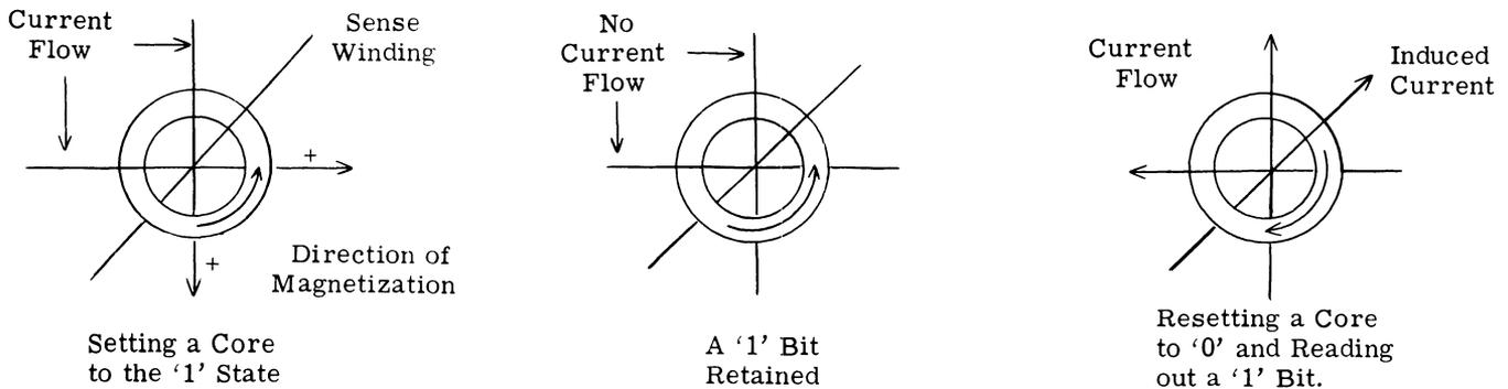
Figure 3-1. Bit Storage in a Ferrite Core
