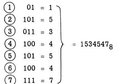
The result of the binary-to-octal conversion is a 7-digit number in place of the longer, less meaningful 20-bit binary word.
