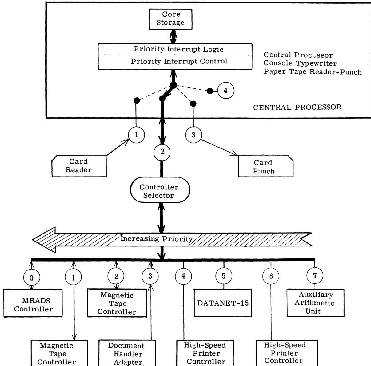
Figure 1-5. Controller Selector Priority
