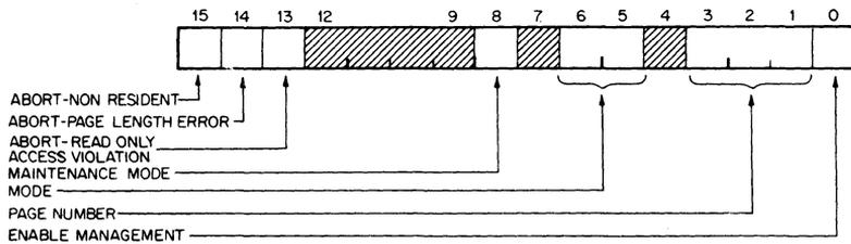
Figure 6-8 Format of Status Register #0 (SR0)
