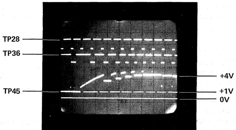
The low on pin 5 is then coupled through transistor Q24 to pin 9 of the phase detector. With pin 9 low, the output at pin 8 is a positive ramp signal with a time constant determined by R6 and C47. This positive ramp is applied through R153,C44 to balance the sum junction of the base of transistor Q24. This positive voltage is also coupled to pin 12 of the VCO to slew up the VCO frequency until the reference frequency matches the tape frequency.
