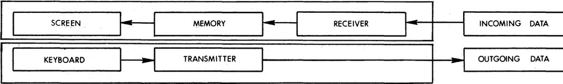
This view is supported by the fact that only two lines are attached to the back of the terminal. Data entered at the keyboard is sent on one line, and data coming in is received through the other line.
