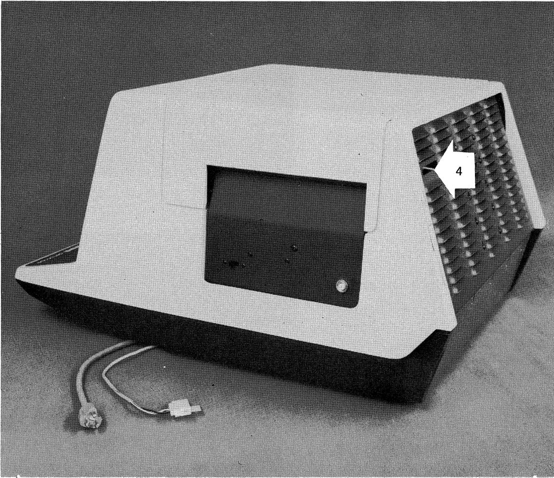
4. Adjust the intensity control for the best image on the screen. This control works like the brightness control on a television set.
