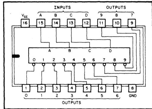
Figure A-1 7442 Package and Logic Diagrams
