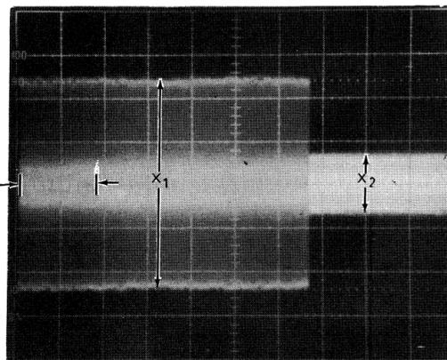
g. Large misalignment. Head inside of CYL 105. Further misalignment reduces amplitude of signal on left side of screen.
