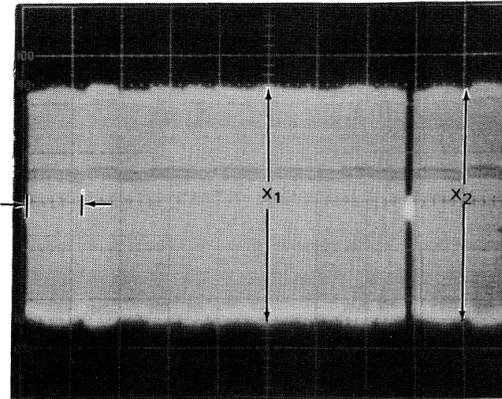
e. Heads slightly misaligned. Larger left amplitude indicates head inside of CYL 105 (toward 106).
