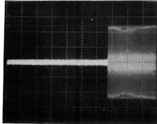
b. Head considerably misaligned. Smaller left amplitude indicates head outside of CYL 105.
