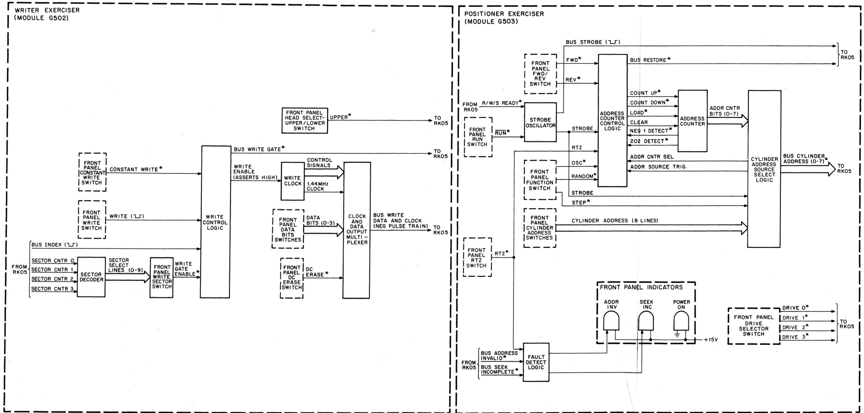
Figure 4-1 RK05 Exerciser Functional Block Diagram
