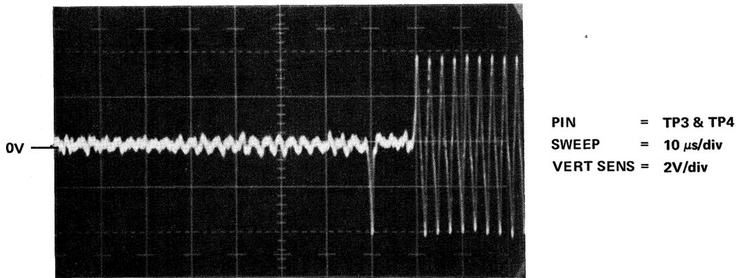
Figure 6-13 Index/Sector Waveform
