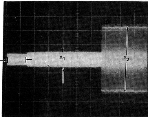
c. Head slightly misaligned. Smaller left amplitude indicates head outside of CYL 105.
