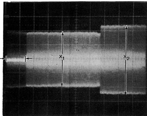
d. Head correctly aligned. Amplitudes are equal.
