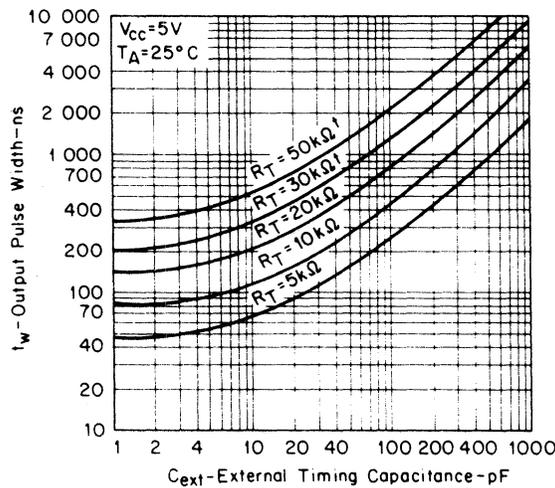
Figure A-3 DEC 74123 IC Output Pulse Width vs. External Timing Capacitance
