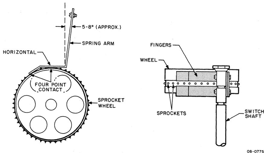
Figure 5-14 Spring Arm Adjustment for PR68D/DA
