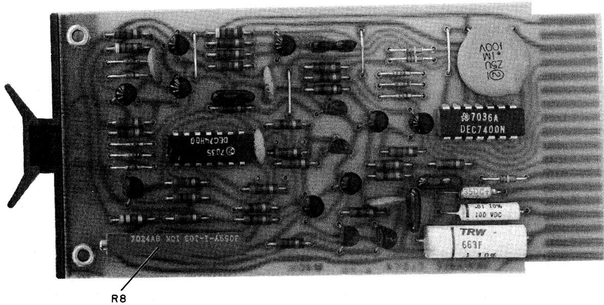
Figure 5-1 M401 Reader Clock Adjustment Location
