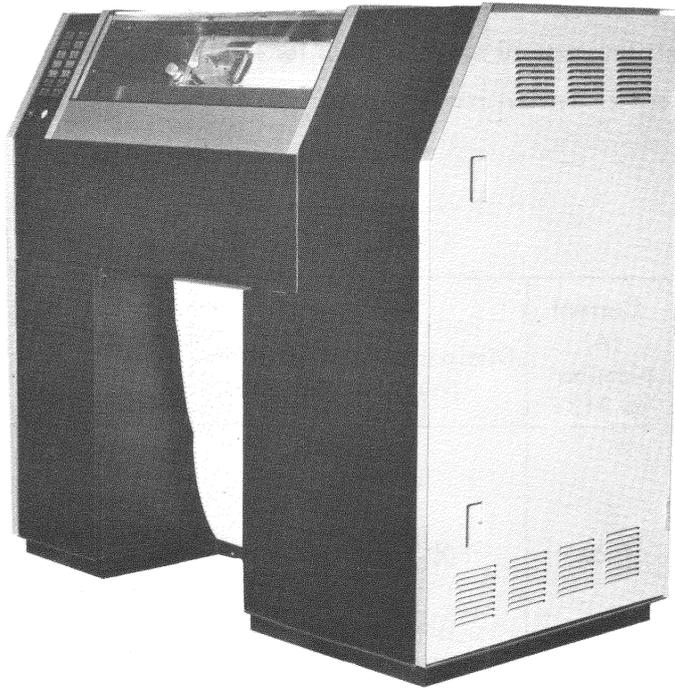
Figure 1-7 LP10B Line Printer
