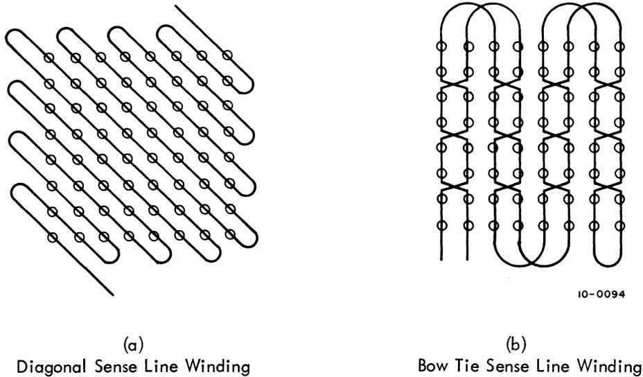
Figure C-10 Sense Winding Configuration
