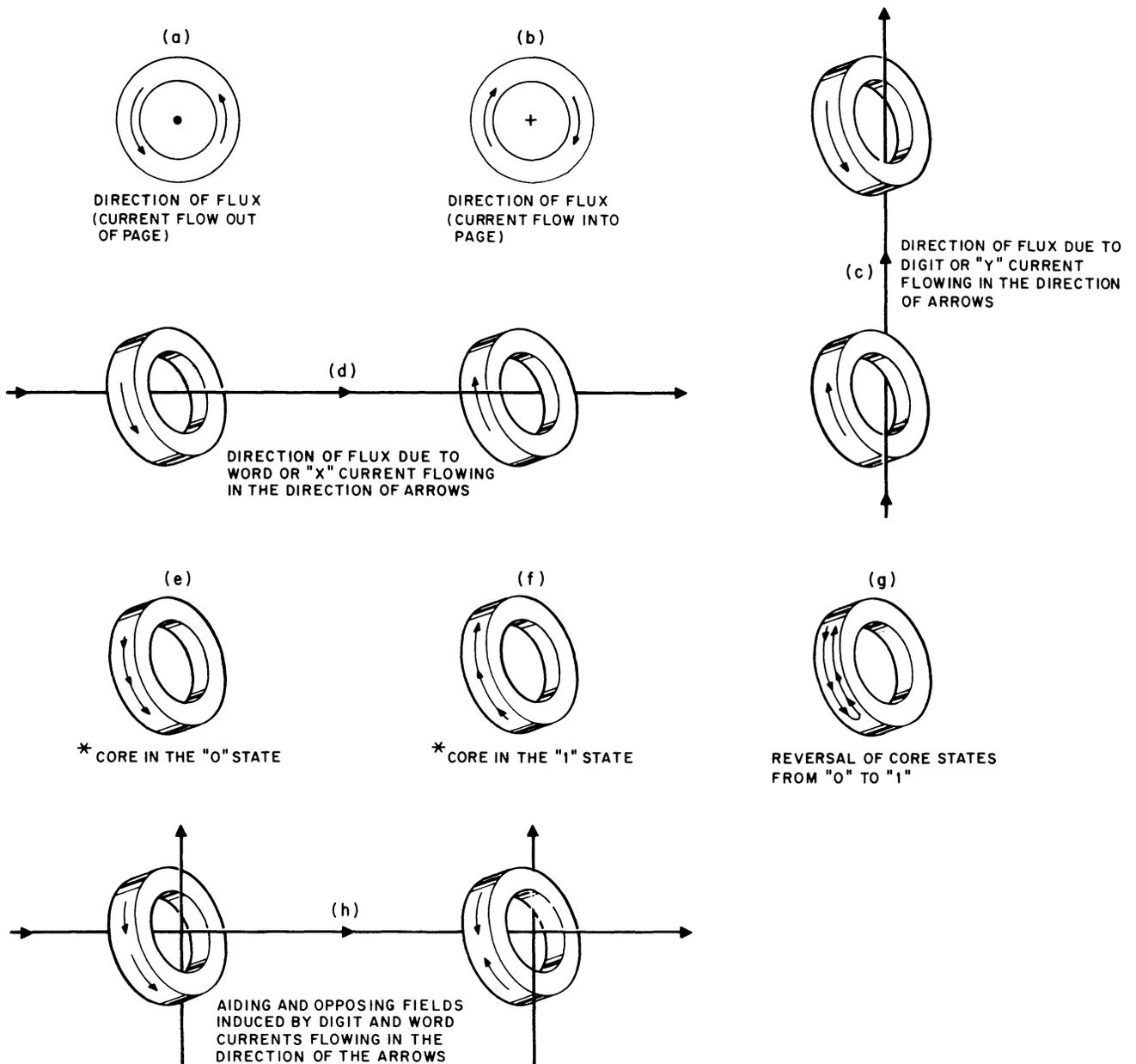
\* THESE CONVENTIONS ARE APPLICABLE TO PLANES 1 AND 3. OPPOSITE CONDITIONS EXIST FOR PLANES 2 AND 4 BECAUSE OF STACK WIRING CONFIGURATION.
