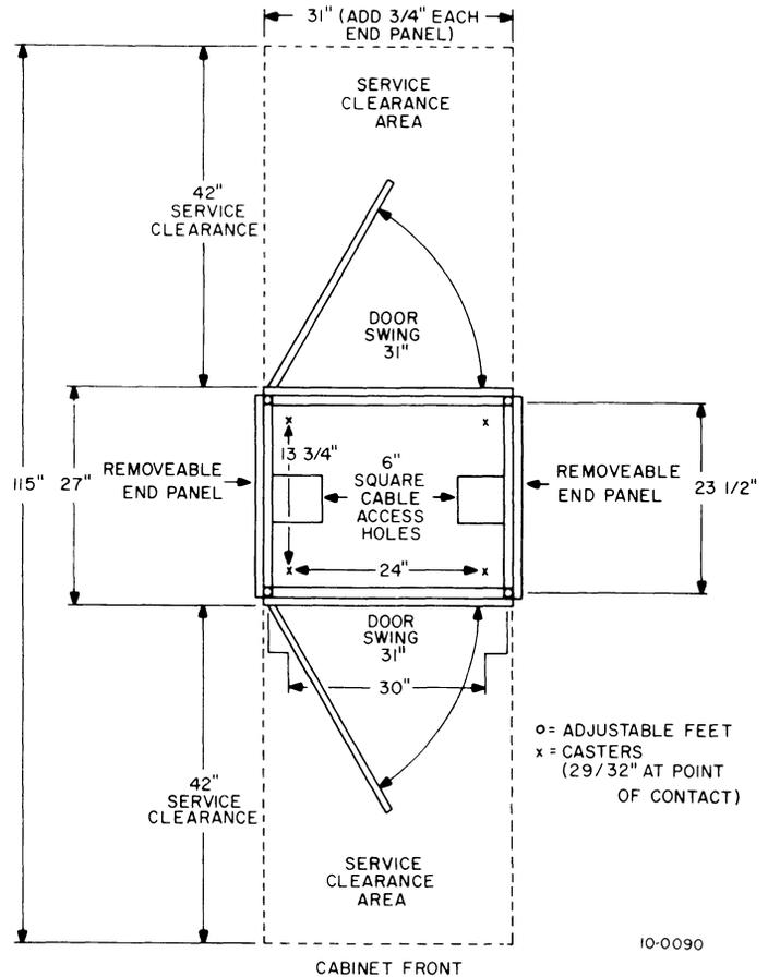
Figure 2-1 MA10/MA10A Core Memory Service Clearances
