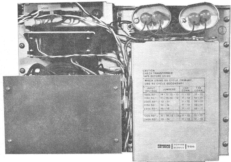
Figure 5-2 Type 706 Power Supply
