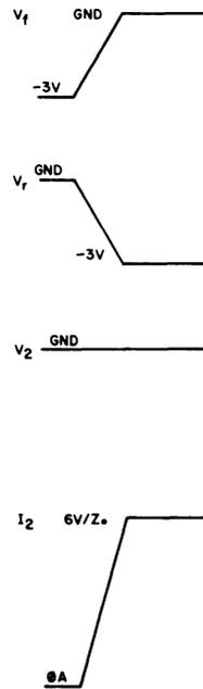
Figure A-3 Waveforms During Reflection
