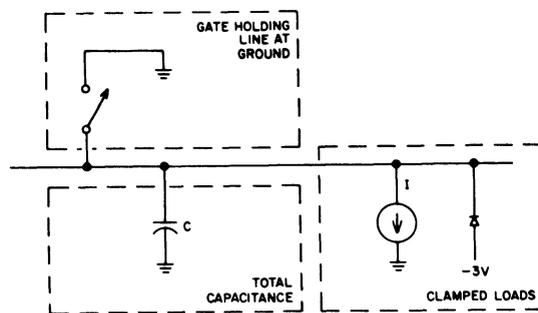
Figure 4-1 Circuit to Estimate Fall Time
