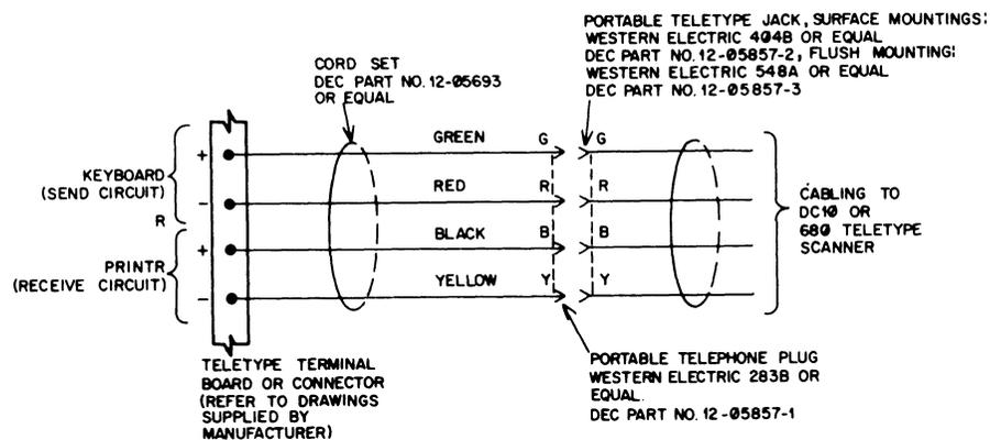
Figure 6-1 20 mA, Full Duplex Terminal Interface
