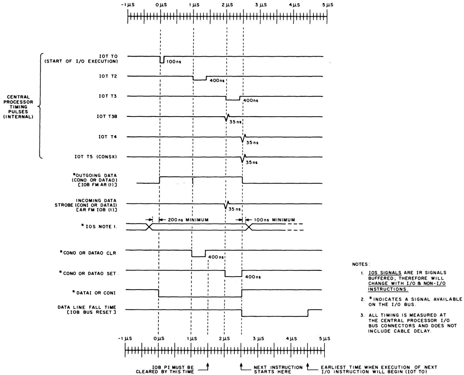
Figure 2-4 I/O Bus Timing
