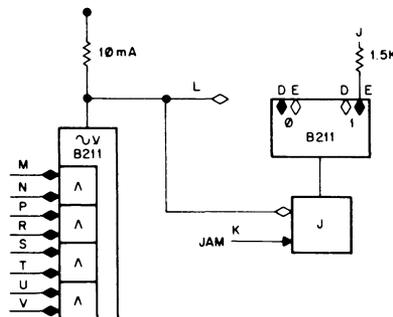
The B211 provides a 2 mA diode gate AND/OR circuit driving a jam flip-flop similar to one half of a B213. It is useful as the memory address register of a PDP-10 memory module.
