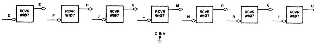
The W107 contains seven identical non-inverting receiver circuits with high-impedance input for buffering signals from the PDP-10 I/O Bus. The W107 is pin compatible with the W500 emitter follower.
