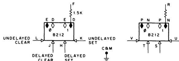
The B212 standard size FLIP CHIP module contains two clear-set flip-flops with buffered outputs and individual delayed and undelayed set and clear inputs.
