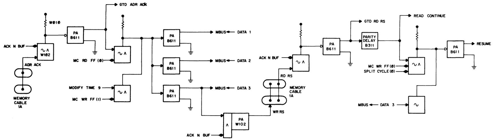
Figure 7-10 Memory Cycle Timing Chain
