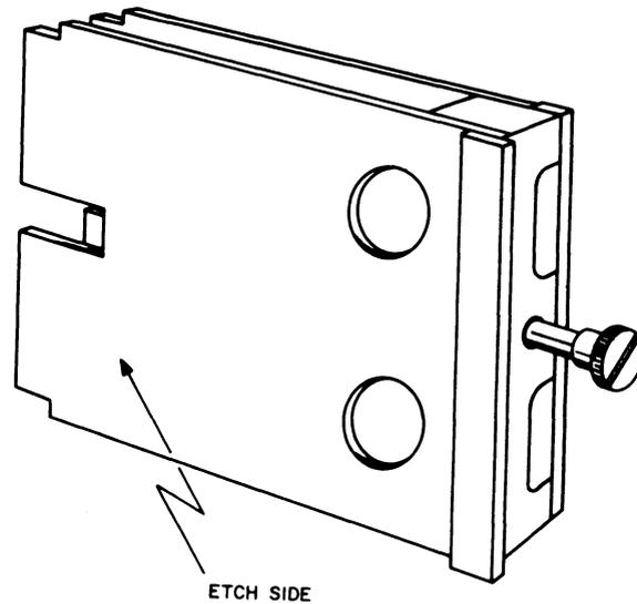
The H351 and H352 are cable connector assemblies suitable for plugging into a H800 connector block equipped with H003 or H004 retaining blocks. They may also be plugged into H800 connector blocks but this will not take advantage of the hold-down screw provided.
