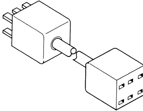
The BC10B Margin Check Cable Assembly is the standard PDP-10 margin check bus cable. It consists of a Cinch-Jones P-306-CCT male plug at one end and Cinch-Jones S-306-CCT female plug at the other end. The cable is arranged as an extension cord; that is, all six pins at one end are connected to the corresponding pins at the other end.
