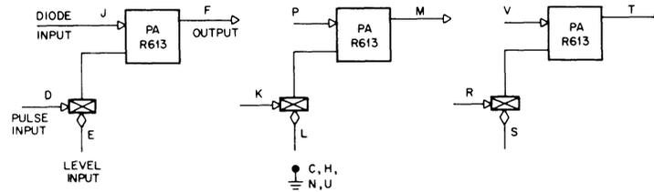
The R613 is pin compatible with and functionally similar to the R603.
