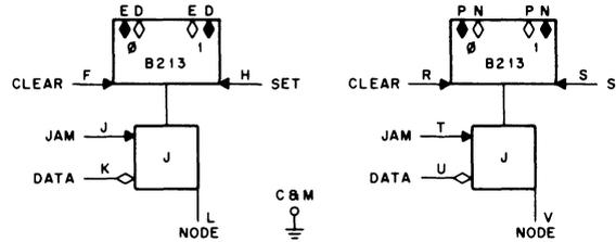
The B213 provides two jam transfer (C-D) flip-flops. It is often used in combination with the B169 diode gate to form a general purpose register. It is also useful as a complementary bus driver.
