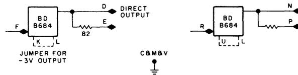
The B684 contains two dual-purpose, non-inverting bus drivers. Each bus driver provides standard DEC levels of -3 V and ground to a large number of diode gates and "inverter base loads" (an inverter base load is a load of -1 mA at -3 V and 60 pF). Alternatively, the bus driver will drive a terminated cable of 90  $\Omega$  characteristic impedance.
