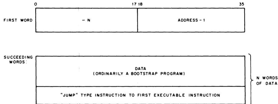
Figure 2-2 Read-In Mode Data Format
