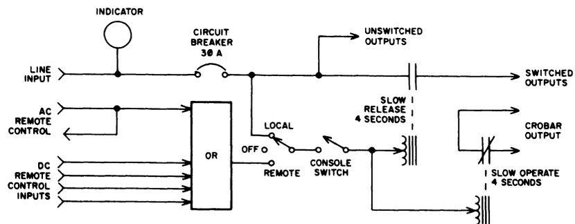
Figure 4-9 844 Power Control Block Diagram
