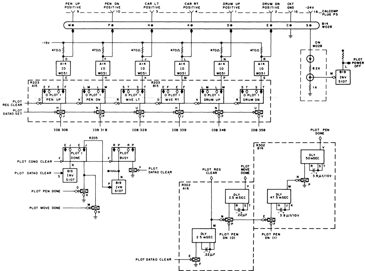
Figure 2-5(c) CalComp Plotter Control
