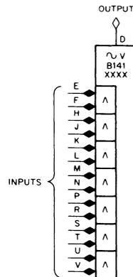
The B141 is a 2 mA diode gate used for performing AND/OR functions and register comparisons. It is typically used for register loading and driving I/O bus data lines. The B141 will operate from standard DEC 35 ns or 40 ns negative pulses, provided that adequate fall times are maintained. It will also operate with standard DEC levels of ground and -3 V. (Pulses 70 ns or wider are considered levels.) Repetition rate may be limited to less than 10 MHz by slow fall times.
