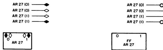
Figure 3-4 Flip-Flop Representation
