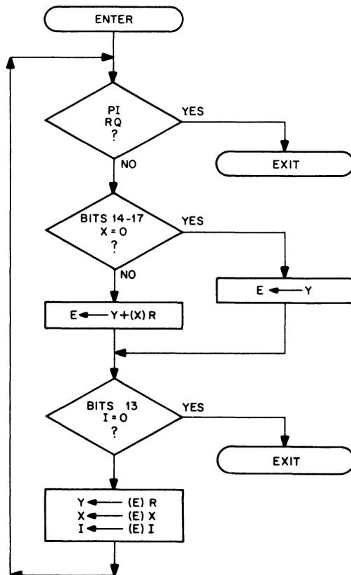
Figure 2-9 Effective Address Calculation
