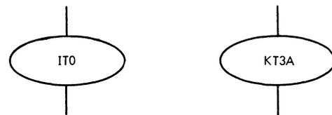
Pulses are named in such a manner that the location of the flow diagram on which it appears is facilitated. Only those pulse amplifiers which are part of the control flow appear as ovals and are named as described below.
