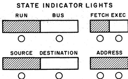
The state indicator lights in the upper right-hand portion of the panel flicker on and off during normal operations. When the ENABLE/HALT switch is in the ENABLE position, and the processor has been STARTed, the RUN light should appear to be on constantly.
