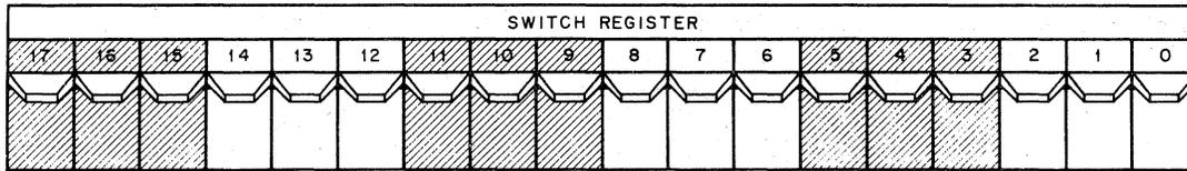
If the positions of the switches in the SWITCH REGISTER represent the address of a location in memory, the address may be loaded into the processor's address register in memory by pressing the LOAD ADDRESS switch (see D.1.4).
