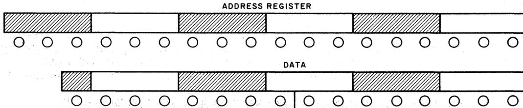
The ADDRESS REGISTER consists of a row of 18 lights divided into six groups of three lights each. Each light position represents a binary digit in an 18-bit word address. When a light is lit, it represents the binary number 1; when a light is off, it represents the binary number 0.
