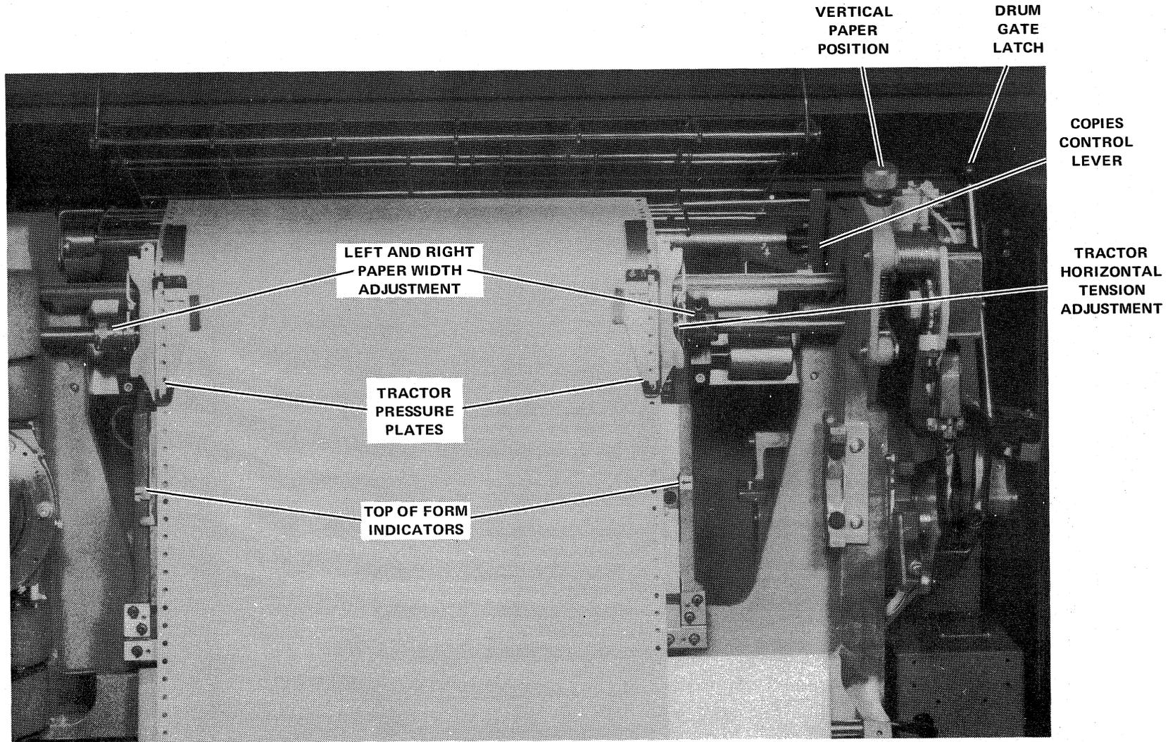
Figure H-4 Mechanical Controls
