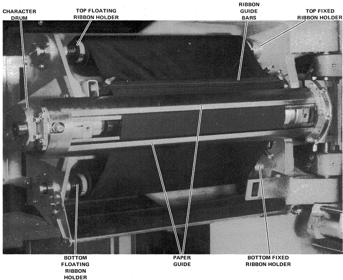
Figure H-5 Drum Gate Ribbon Installation
