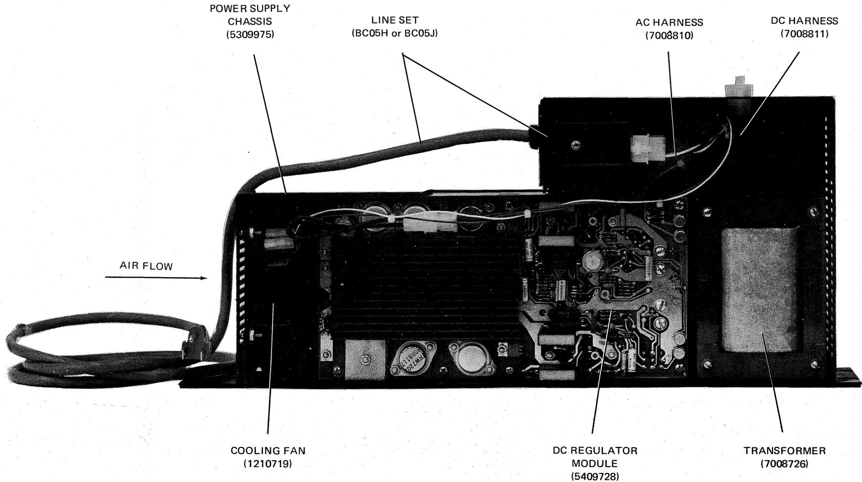
Figure 1-1 H740D Power Supply Components
