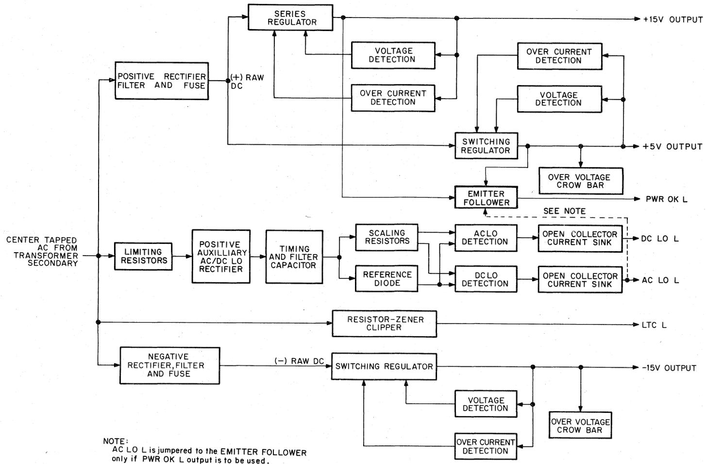
Figure 3-5 dc Regulator Module, Block Diagram
