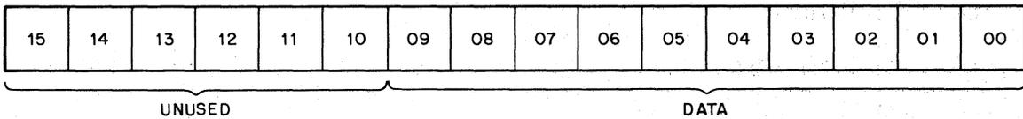
Figure 4-5 X and Y Buffer Registers
