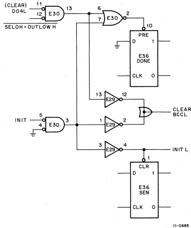
Figure 3-11 Clear and Initialize Control Signals, Logic Diagram
