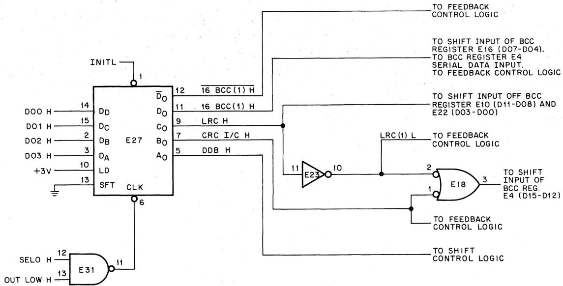
Figure 3-10 Mode Selection Control Signals, Logic Diagram
