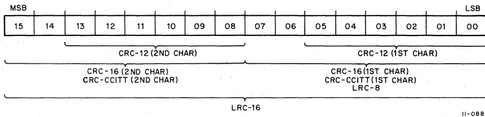
Figure 3-9 BCC Register Format
