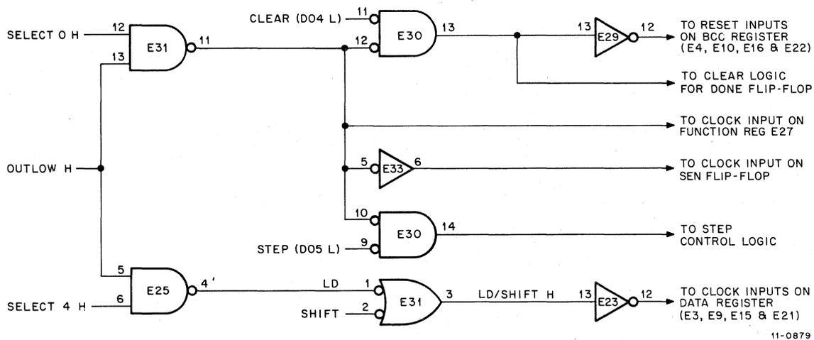
Figure 3-5 Control Signals Generated During DATO (Write) Operation, Logic Diagram
