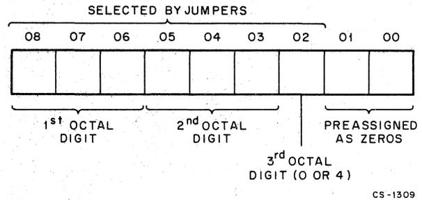
Figure 2-2 DECKit11-D Interrupt Vector Address Select Format
