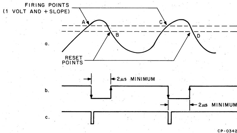
Figure 3-4 Schmitt Trigger Firing
