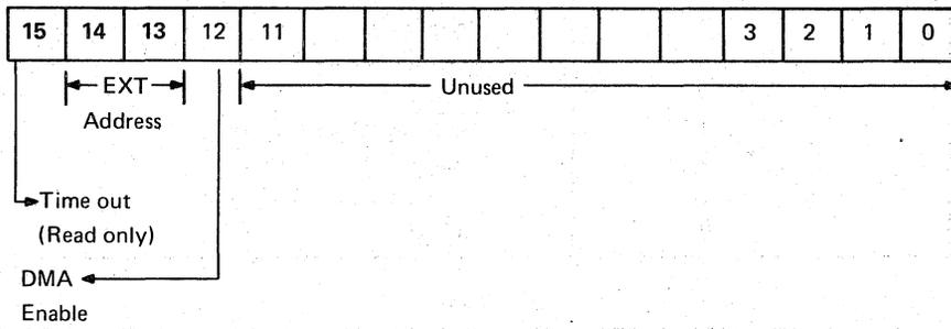
**DMA Current Address Register**
