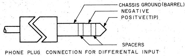
Figure 3-3 Input or Output Phone Jack Connections
