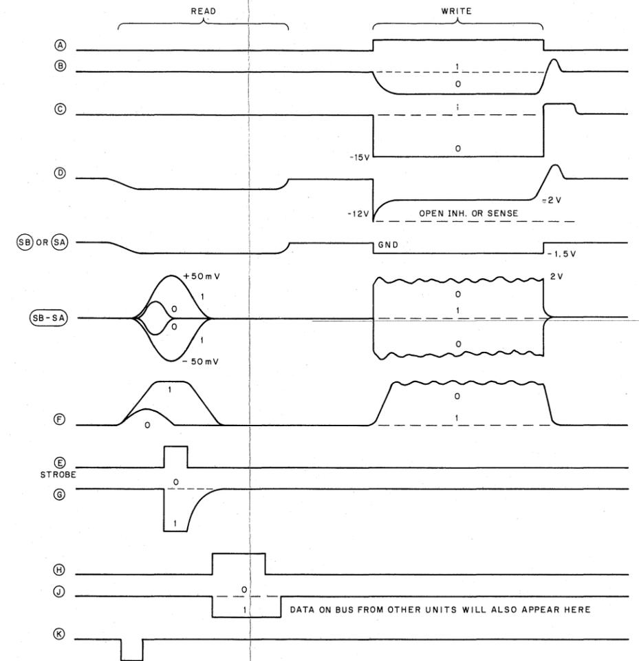
Figure 3-33 MM11-L Sense/Inhibit Waveforms
