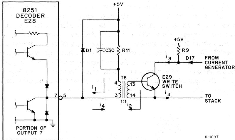
Figure 3-15 Switch or Driver Base Drive Circuit
