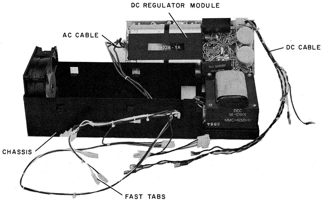
With DC Regulator Module Removed
