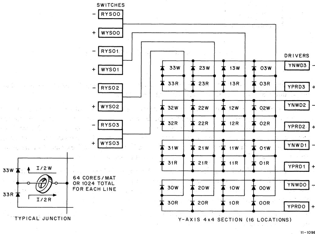
Figure 3-16 Y-Line Selection Stack Diode Matrix
