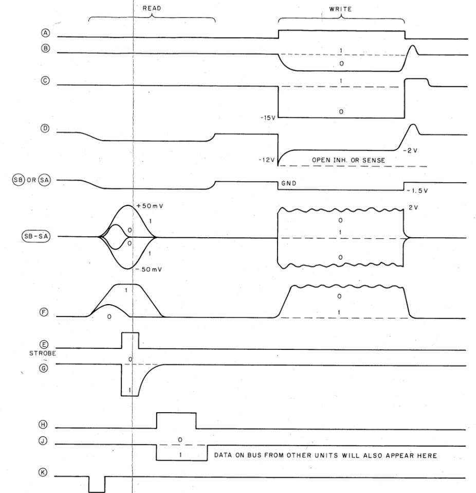
Figure 3-3 MM11-L Sense/Inhibit Waveforms
