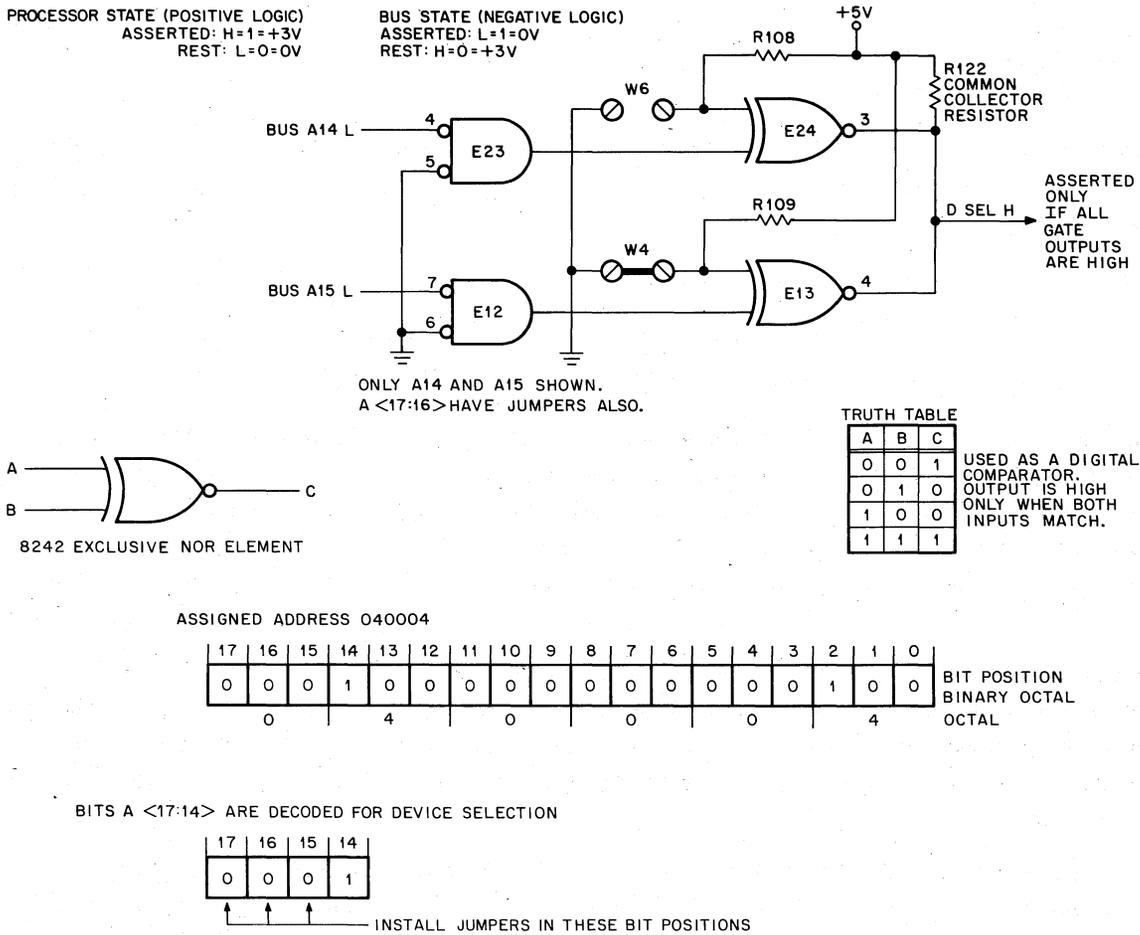
Figure 2-7 Jumper Configuration for a Specific Memory Address
