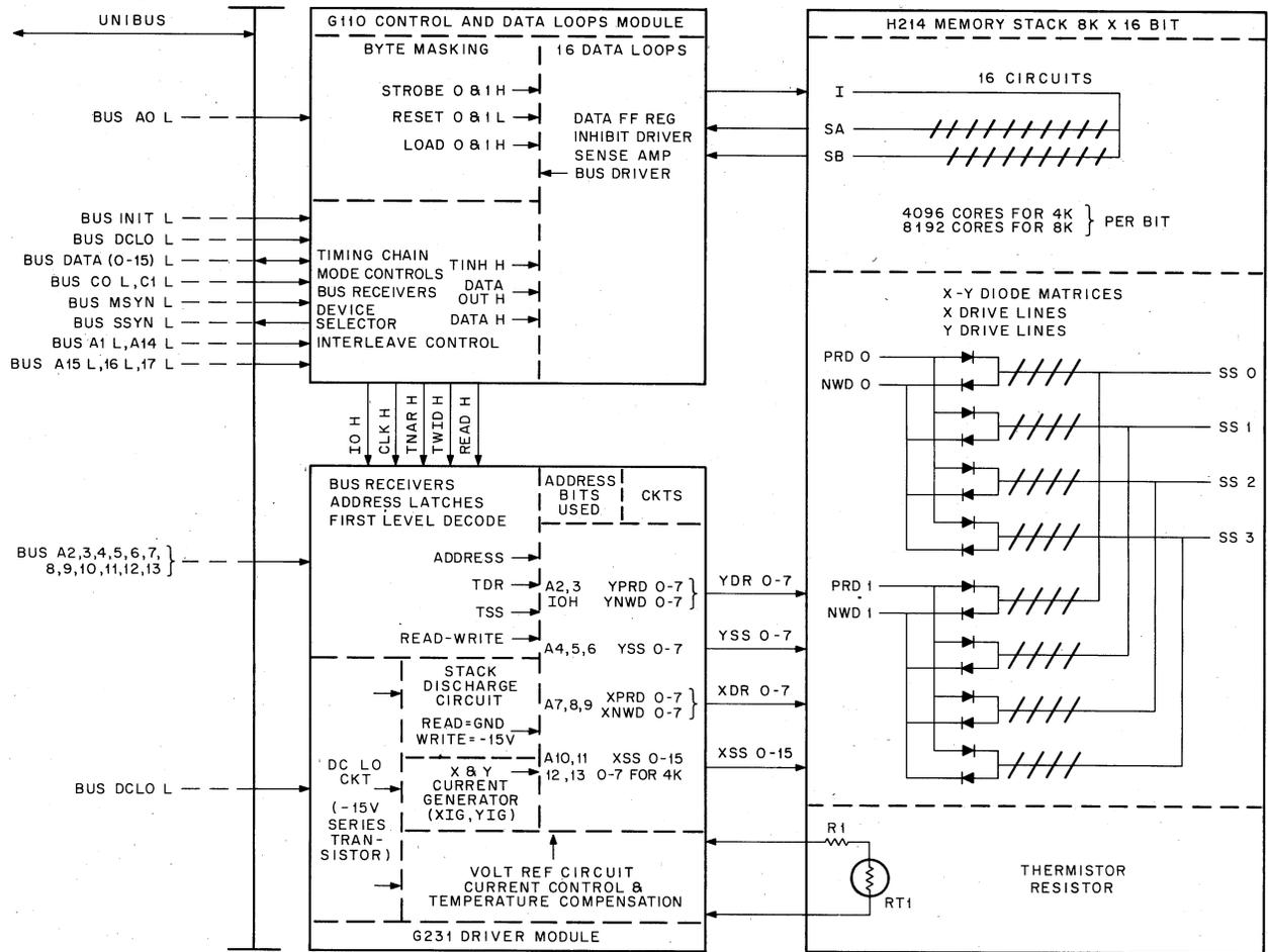
Figure 1-5 MM11-L Memory Block Diagram
