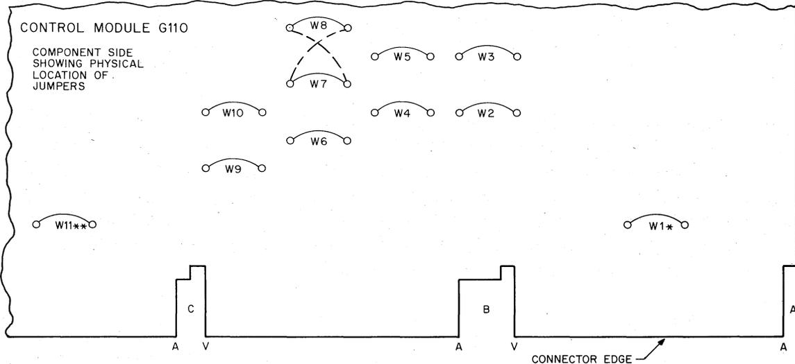
\* Jumper W1 is for test purposes only. It must be installed for normal operation.
