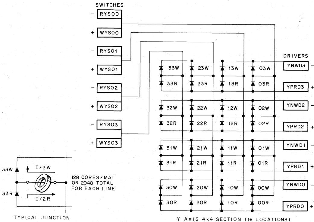
Figure 2-12 Y Line Selection Stack Diode Matrix
