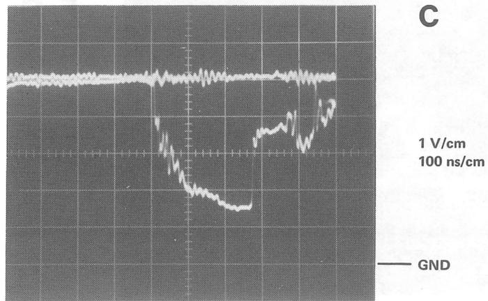
Figure 5-7 Sense Inhibit Module Waveforms (Sheet 1 of 4)
