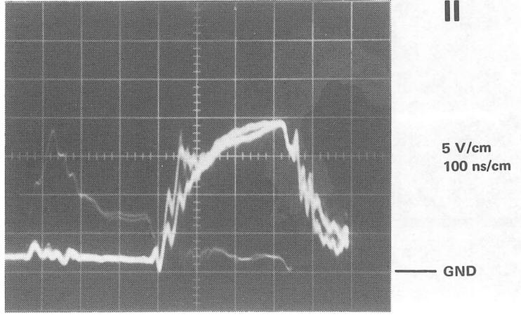
Figure 5-9 Drive Module Waveforms (Sheet 3 of 3)
