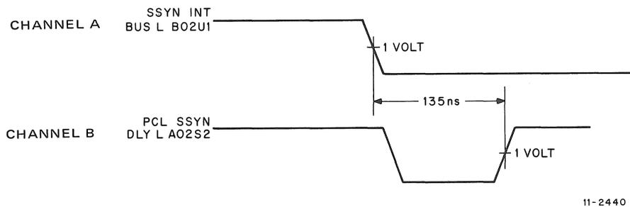
Figure 5-4 SSYN DLY L Timing Waveform
