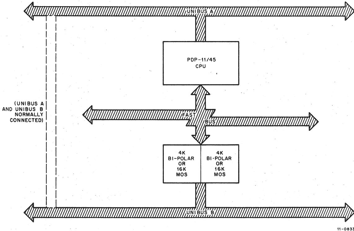
Figure 2-1 Semiconductor Memory Configuration within PDP-11/45 Systems
