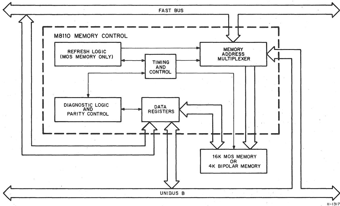
Figure 1-2 MS11 Semiconductor Memory Control Module, Block Diagram
