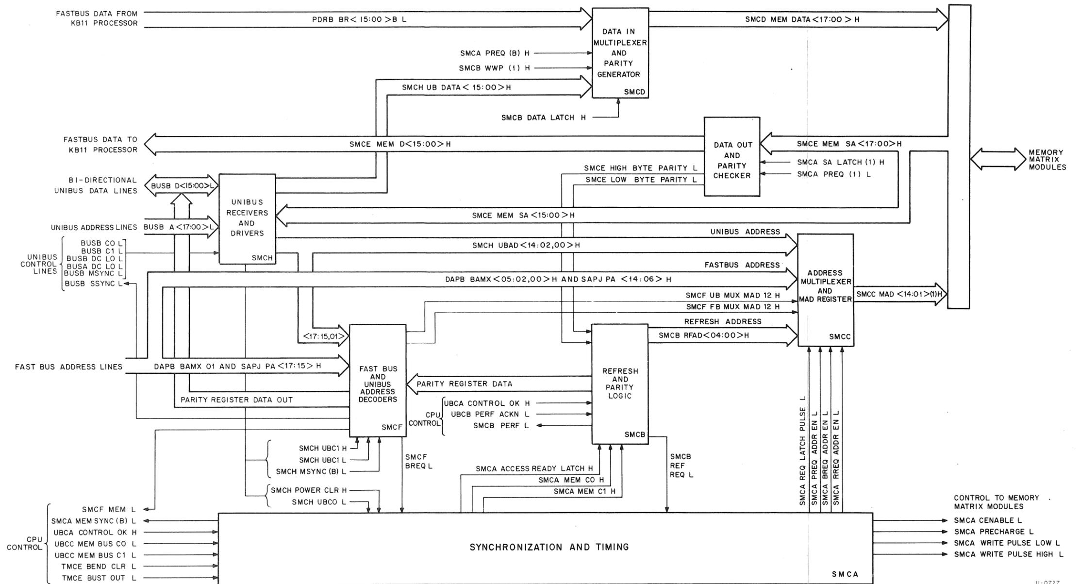
Figure 3-3 M8110 Semiconductor Memory Control Module, Block Diagram
