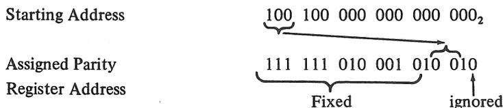
**3.4.7.2 Parity Register** – This register consists of three 74H74 D-Type flip-flops shown on drawing SMCB: parity error (PE), write wrong parity (WWP), and error indication enable (EIE). Table 3-12 lists their bit assignments and functions.
