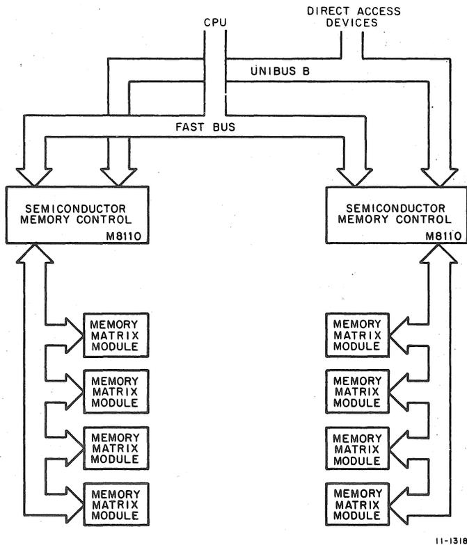
Figure 1-1 MS11 Semiconductor Memory System, Block Diagram
