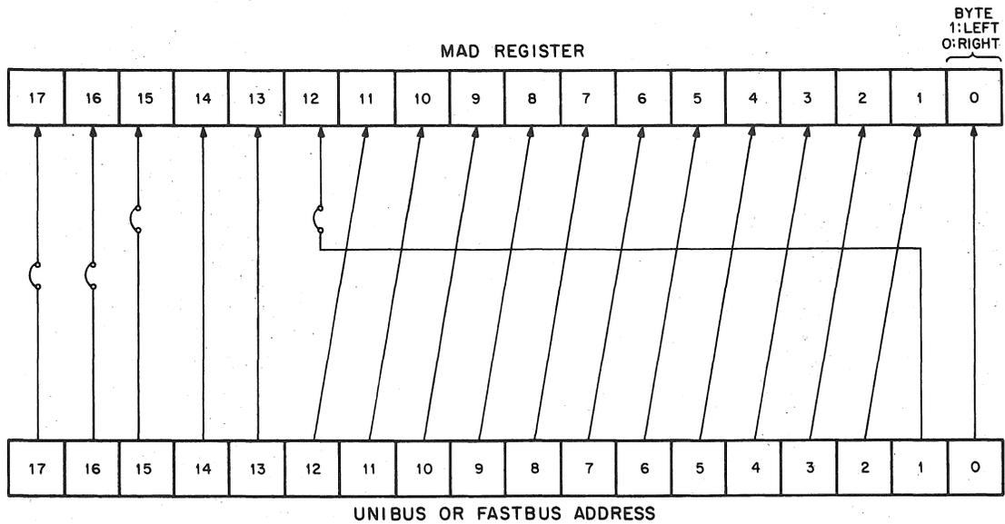
Figure 2-7 Semiconductor Memory Address Mapping
