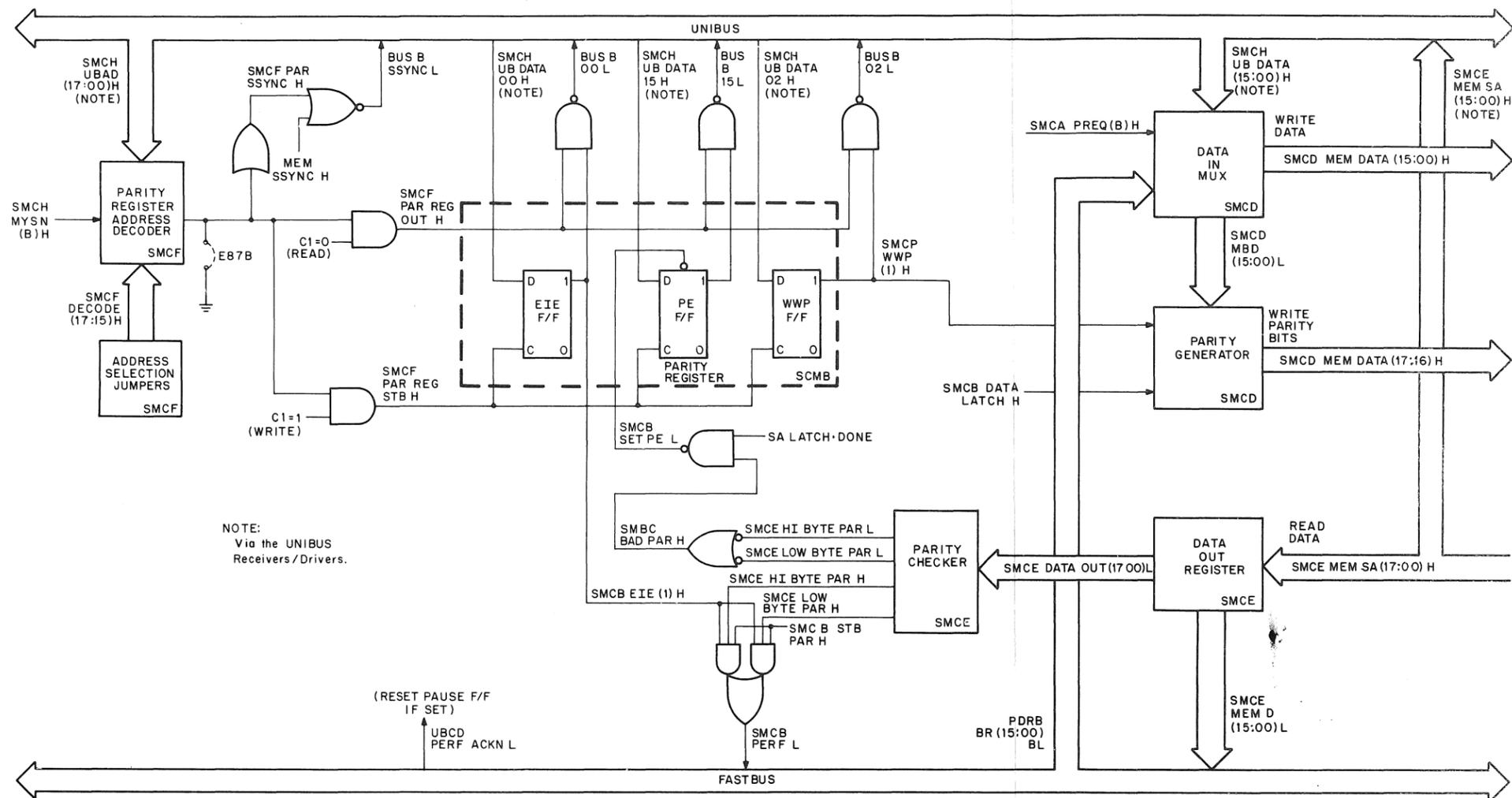
Figure 3-18 Parity Logic, Block Diagram
