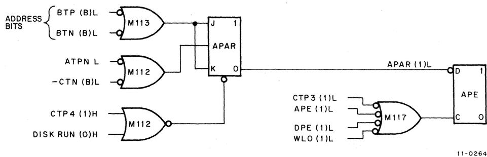
Figure 4-25 Address Parity Error
