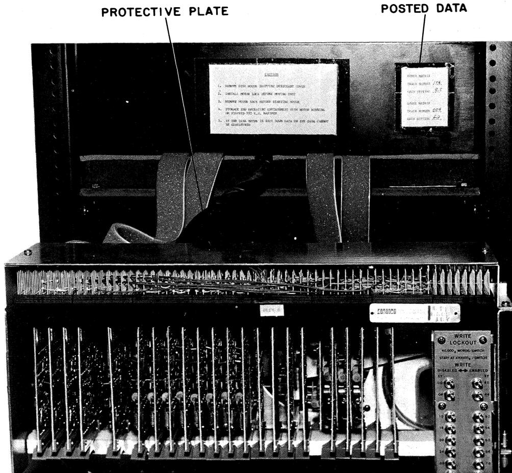
Figure 7-5 RS11 Electronics Showing Posted Data
