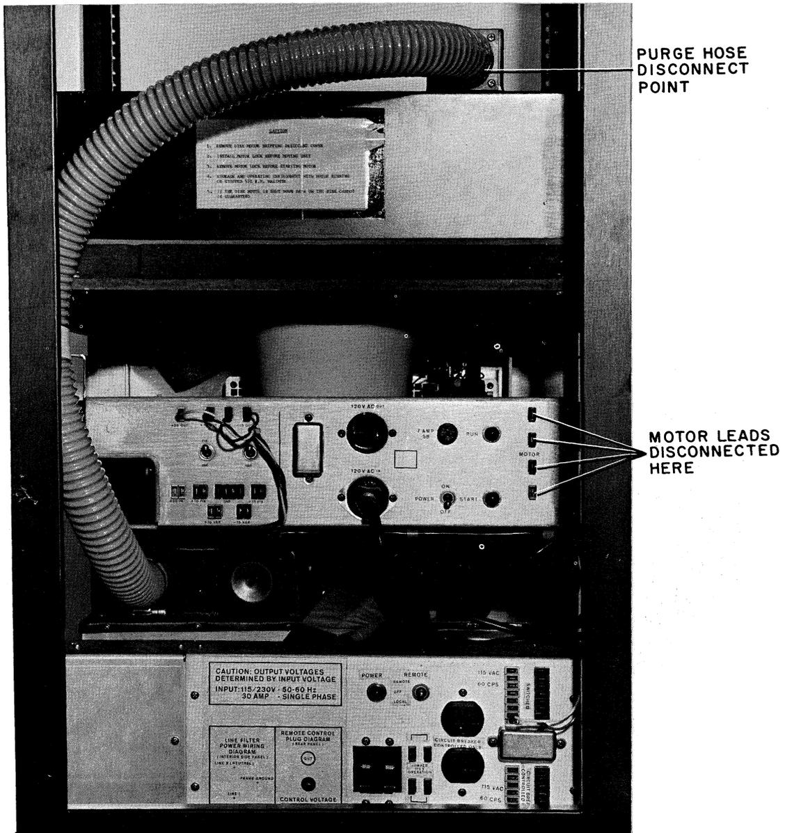
Figure 7-8 Disconnecting Motor Leads and Purge Hose
