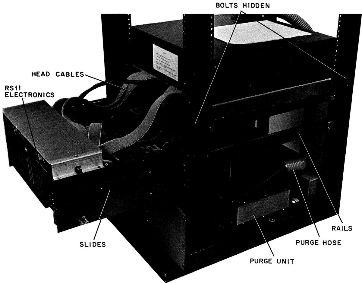
Figure 7-7 Removing the Disk Assembly from the Cabinet
