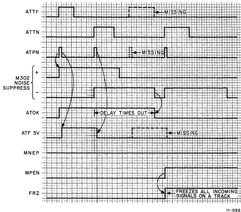
Figure 4-10 A Track Error Detection, Timing Diagram
