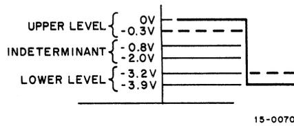
Figure 5-1 Voltage Spectrum of Negative Logic Systems
