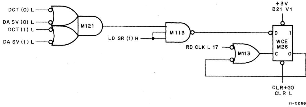
Figure 4-23 Write Check Error
