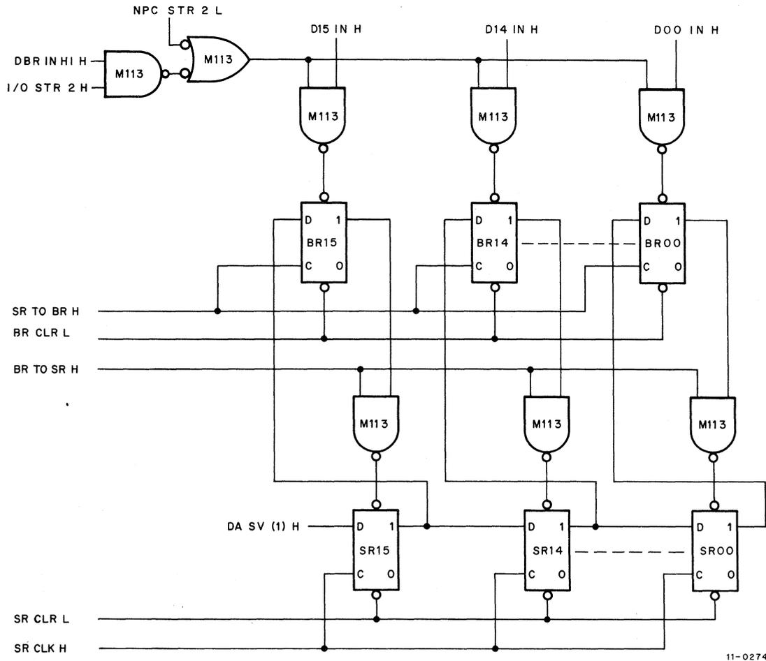
Figure 4-20 Buffer Register and Shift Register Interconnections
