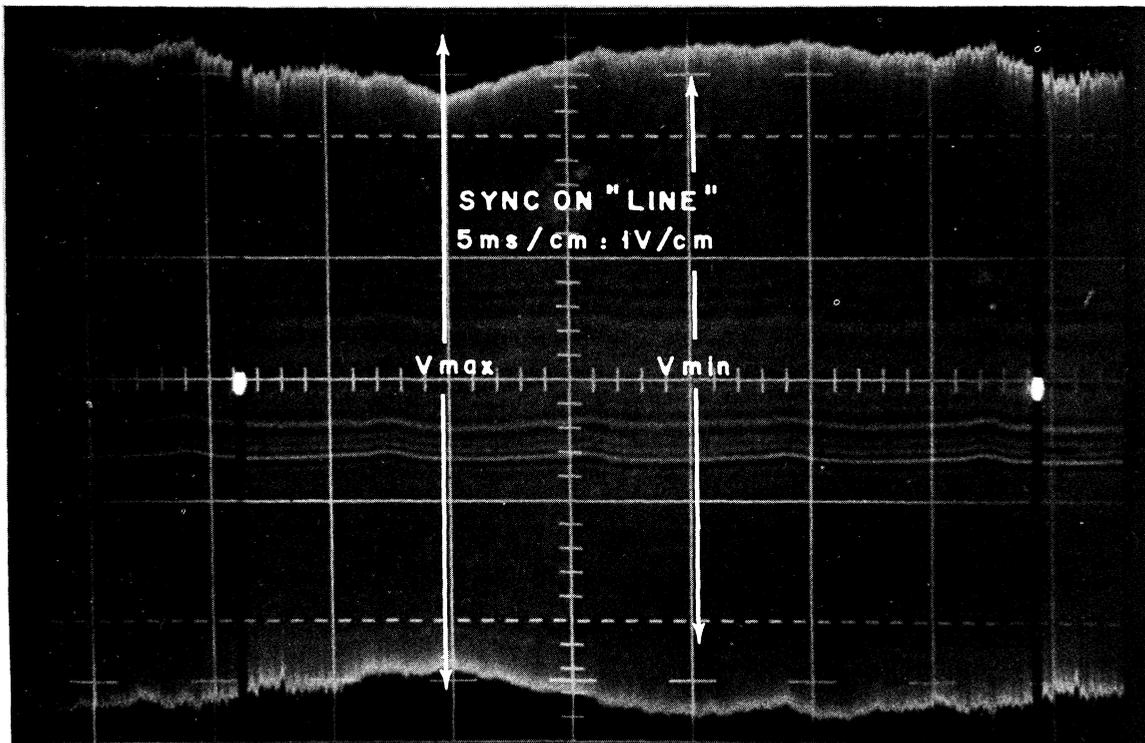
Figure 7-18 Surface Modulation
