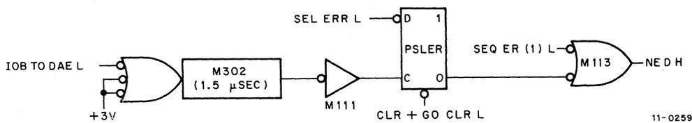
Figure 4-29 Nonexistent Disk by Program Selector Error
