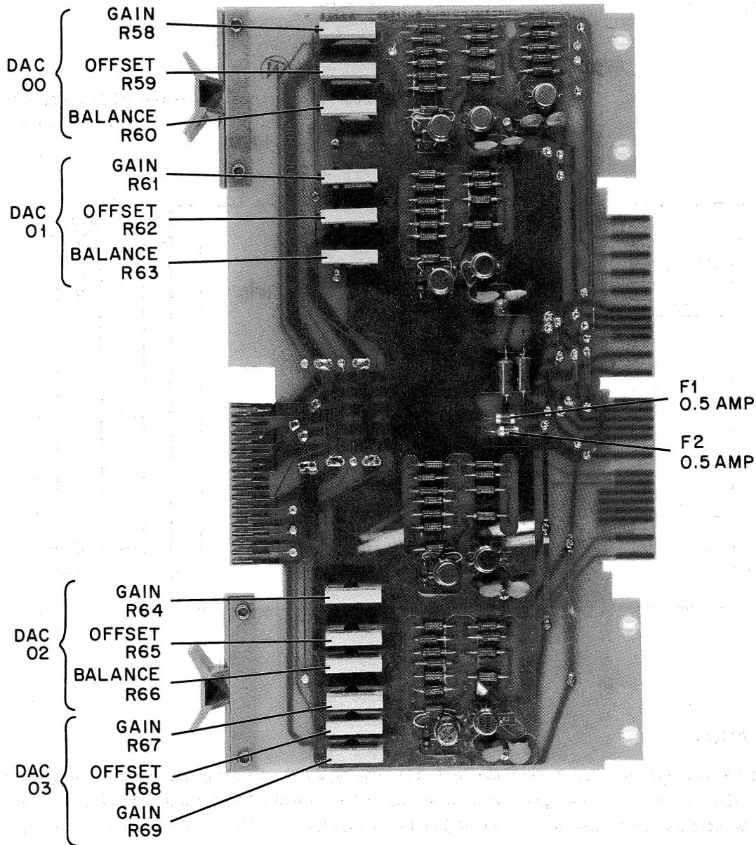
Figure 4-62 Location of Adjustments and Fuses (A236)
