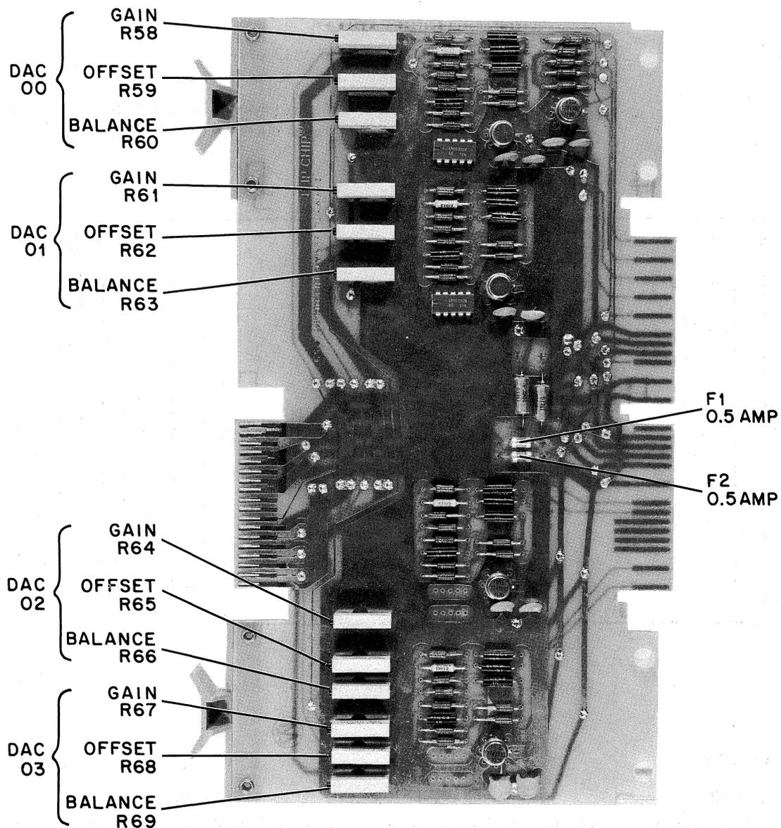
Figure 4-60 Location of Adjustments and Fuses (A235)
