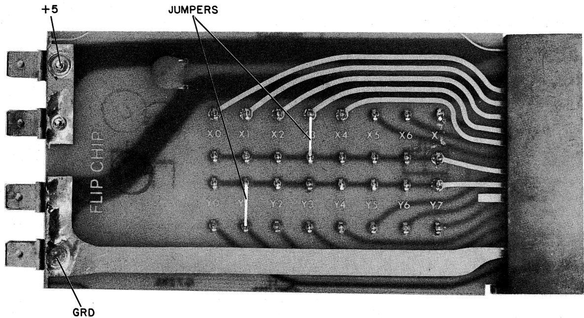
Figure 4-6 G729 Address Jumper Module
