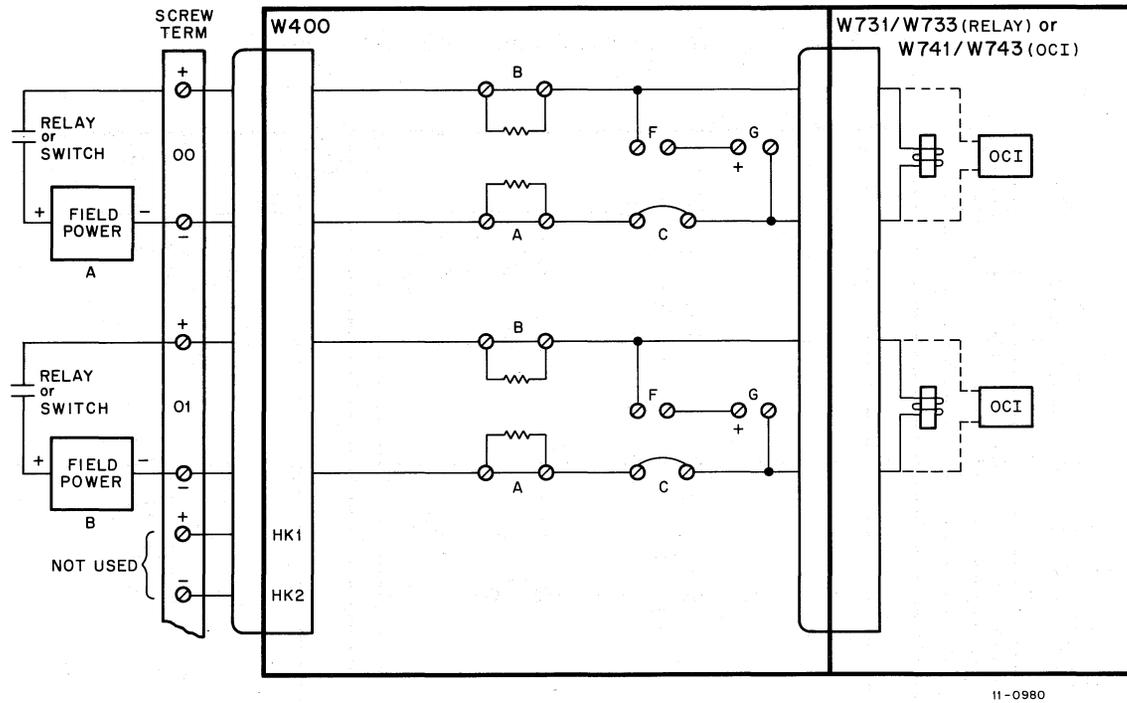
Figure 4-32 Isolated Power for Contact Sensing, Wiring Diagram
