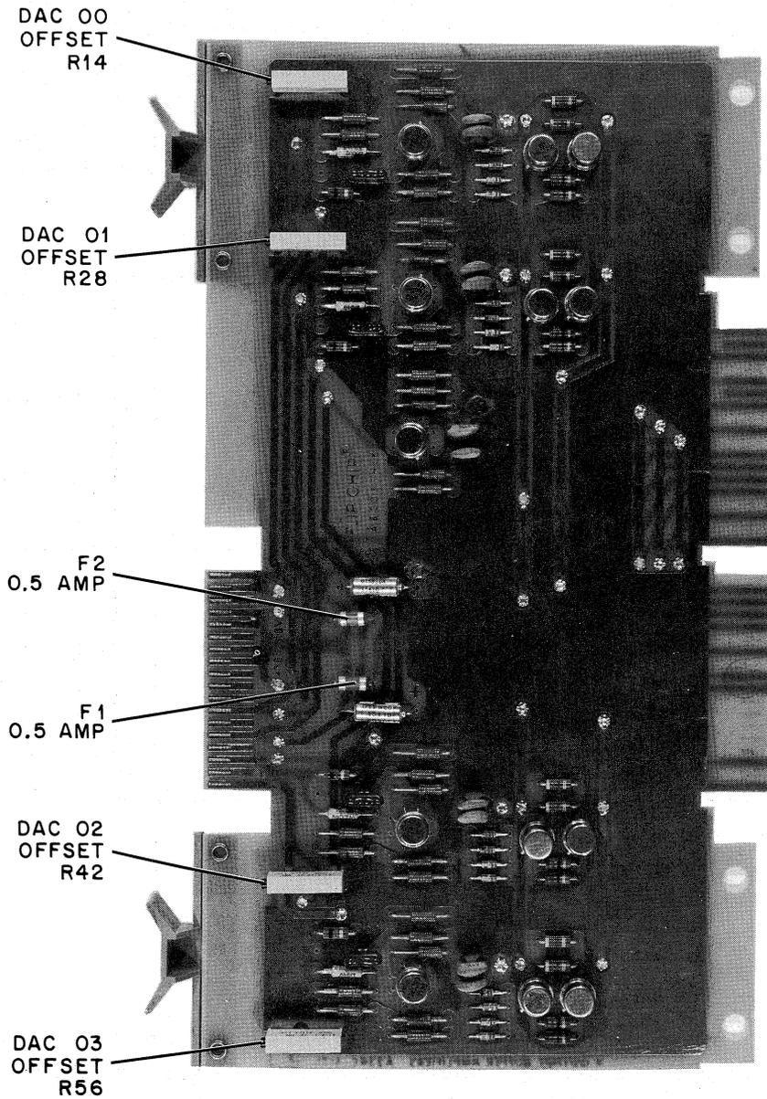
Figure 4-58 Location of Adjustments and Fuses (A234)
