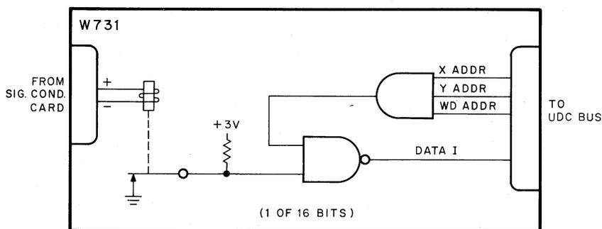
Figure 4-9 Simplified Schematic Diagram (W731)
