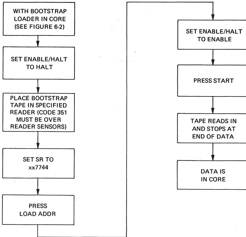
Figure 6-3 Loading Bootstrap Tapes Into Core
