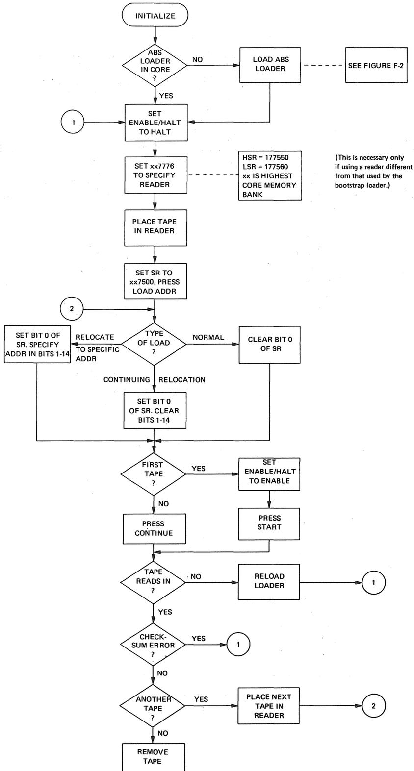
Figure F-3 Loading with the Absolute Loader
