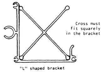
Figure 3-2 Inserting Cross in Roll Paper
