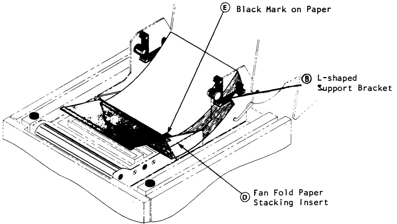
Figure 3-11 Position of Stack for Fanfold Operation
