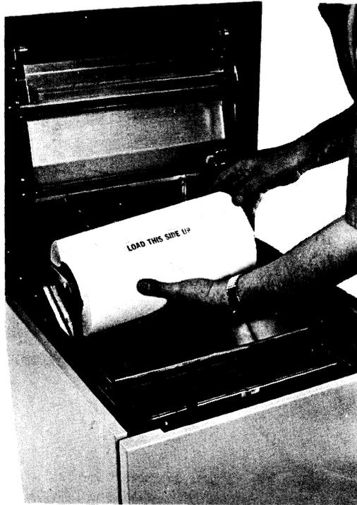
Figure 3-3 Inserting Roll Paper
