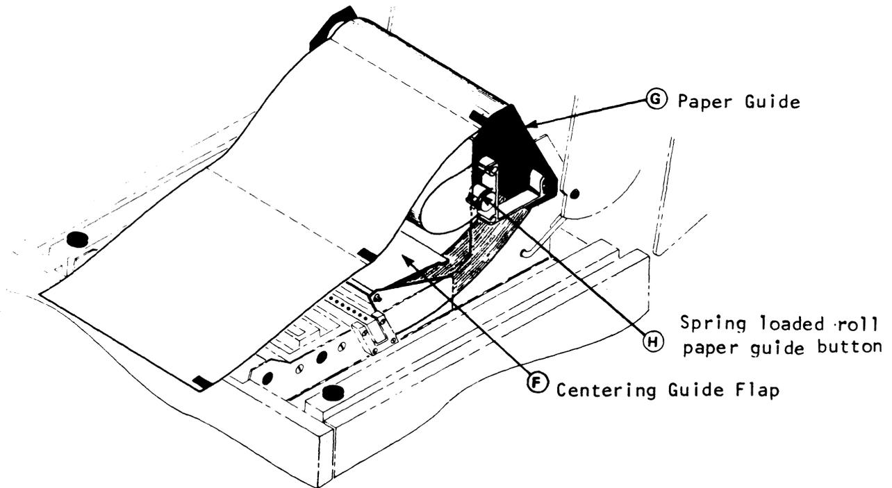
Figure 3-12 Loading Paper over the Paper Guide Assembly
