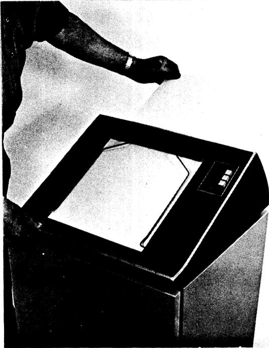
Figure 3-14 Paper Loaded and Top Casting Closed
