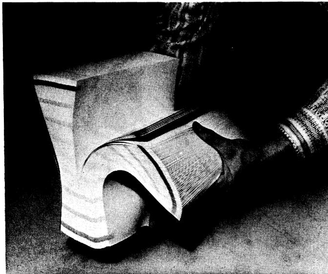
Figure 3-10 ‘Fan’ the Paper to Loosen the Sheets
