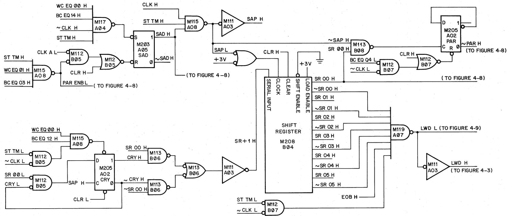
Figure 4-7 Block Address Shift Register Logic Diagram
