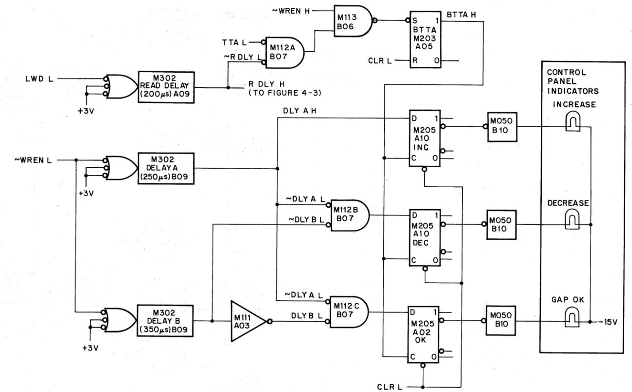
Figure 4-9 Gap Detect Logic Diagram
