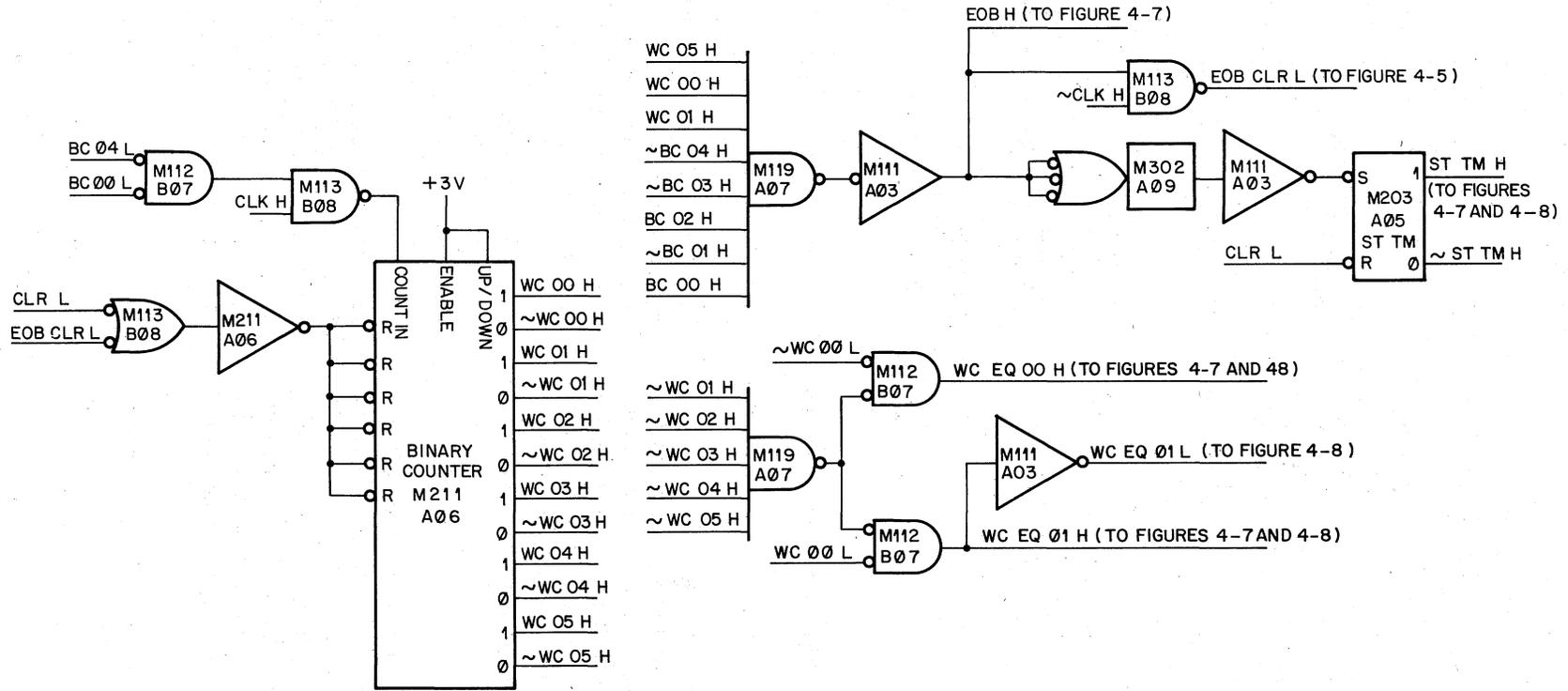
Figure 4-6 Word Counter and Word Count Decode Logic Diagram
